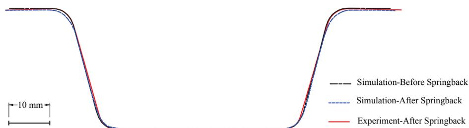
Figure 2.13.: Comparison of the obtained final shapes before and after spring-back from simulation with the final shapes after spring-back from experiment at wider opening end. The numerical result agrees well with the experimental data.
