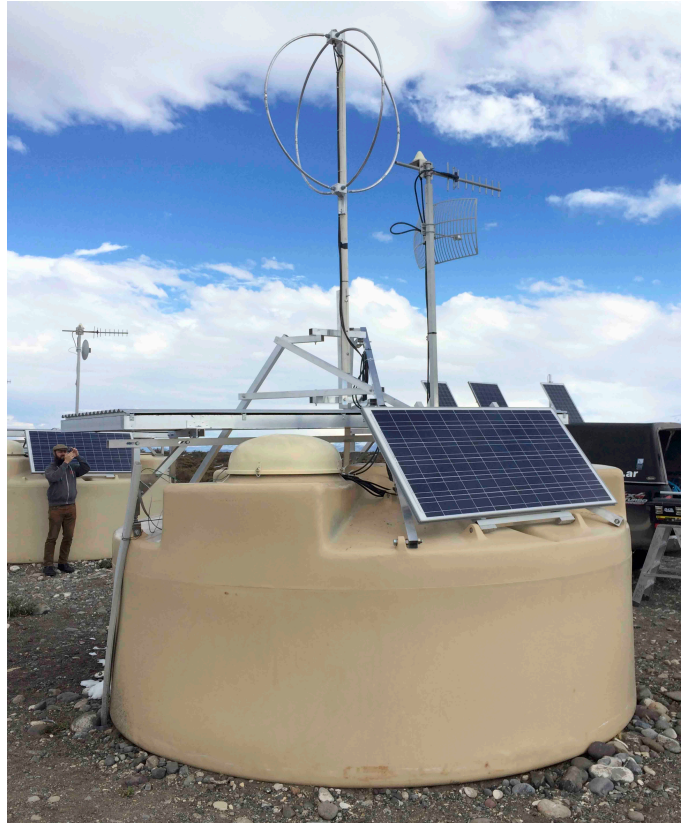
Figure 2.14: Photograph of the upgraded SD station equipped with a scintillator as well as an antenna on top of the tank (from [89]).
