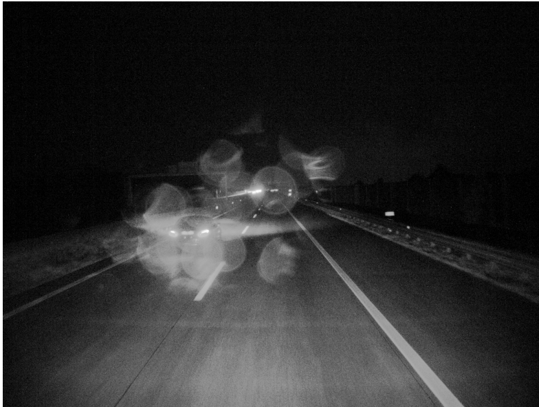
Figure 3.4.: Raindrops might cause drops on the windshield, which break the light in possibly unpredictable ways
