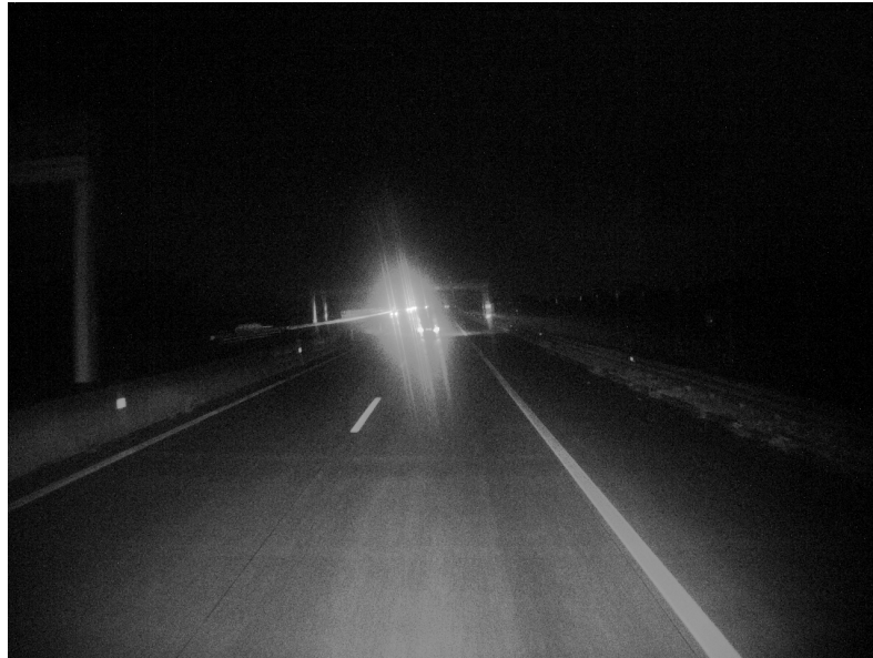
Figure 3.5.: Different light intensities can lead to more or less blooming in the image
