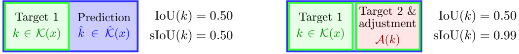
Figure 3: Illustration of the ordinary component-wise intersection over union (IoU) and the adjusted one (sIoU). In both examples above, the prediction \hat{k} (blue rectangle) is the same but covers different targets (green rectangles). On the left, both IoU and sIoU yield the same score. On the right, IoU punishes the prediction as it does not cover each object precisely. By contrast, sIoU checks how much the predictions cover the ground-truth regions, independently of whether prediction/ground truth belongs to a single or multiple objects. In automated driving, it is more important to detect all anomalous regions (whether they belong to single or multiple objects), rather than to detect each object precisely. Since two targets are separated by at least one pixel, IoU = sIoU = 1 if and only if the prediction covers one target perfectly.
