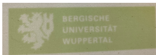
Figure 4.8: Photograph of the bifacial ACEL-device placed on a computer screen which displays the logo of the University of Wuppertal. The device is clearly translucent with a high degree of haze. Published in [104].
