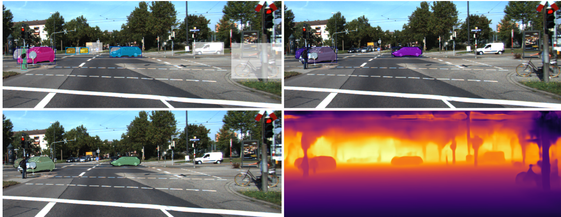
Figure 5.1: Top left : Ground truth image with ignored regions (white). The bounding boxes drawn around the instances represent the class, red denotes pedestrians and blue cars. The cyan colored bounding boxes highlight non-detected instances. Top right : Instance segmentation. Bottom left : A visualization of the calculated instance-wise IoU of prediction and ground truth. Green color corresponds to high IoU values. Bottom right : Depth estimation map.
