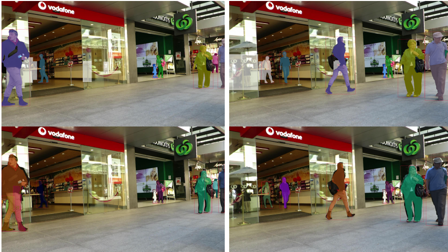
Figure 4.4: Two frames of the MOT dataset. Between both frames is a time gap of two seconds, i.e., 60 frames. Top : Ground truth with ignored regions (white). Bottom : Instance segmentation obtained by the Mask R-CNN. Each color correspond to an instance ID.
