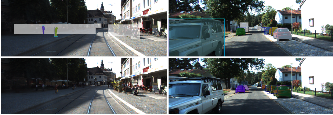
Figure 4.14: Top : Ground truth of two different images with ignored regions (white). Bottom : Instance segmentation obtained by the YOLACT network resulting in non-detected ground truth instances, i.e., false negatives (cyan colored bounding box at the top).
