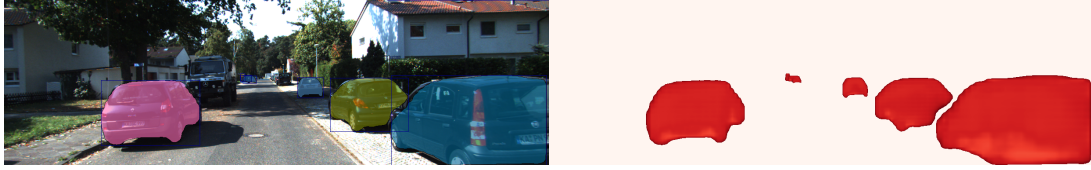
Figure 4.6: Left : Instance segmentation predicted by the Mask R-CNN. Right : Corresponding pixel-wise entropy. The missing predictions of the cars are located in ignored regions and for this reason, not considered.
