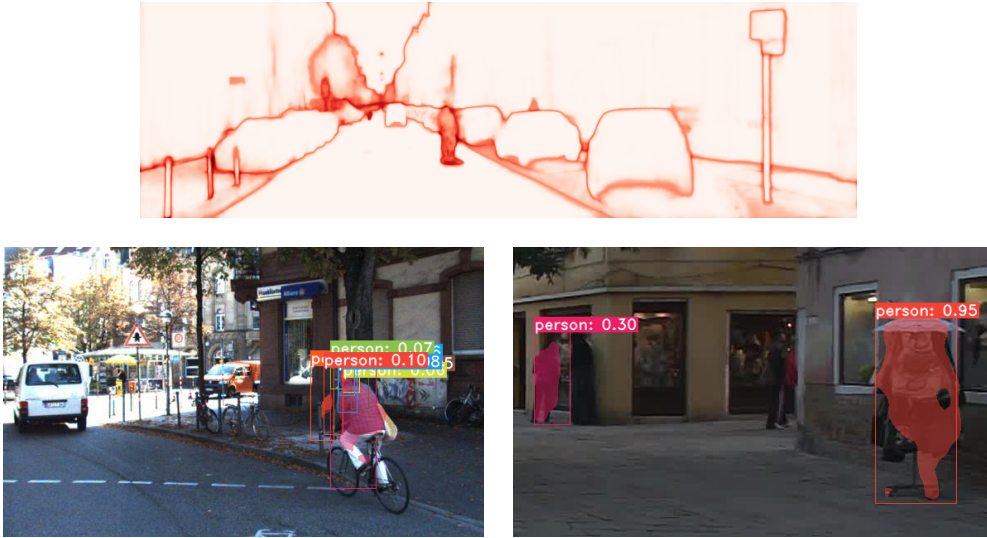
Figure 2.16: Top : Pixel-wise entropy heatmap obtained by the softmax output of a semantic segmentation network. Bottom : Two predictions of an instance segmentation network.
