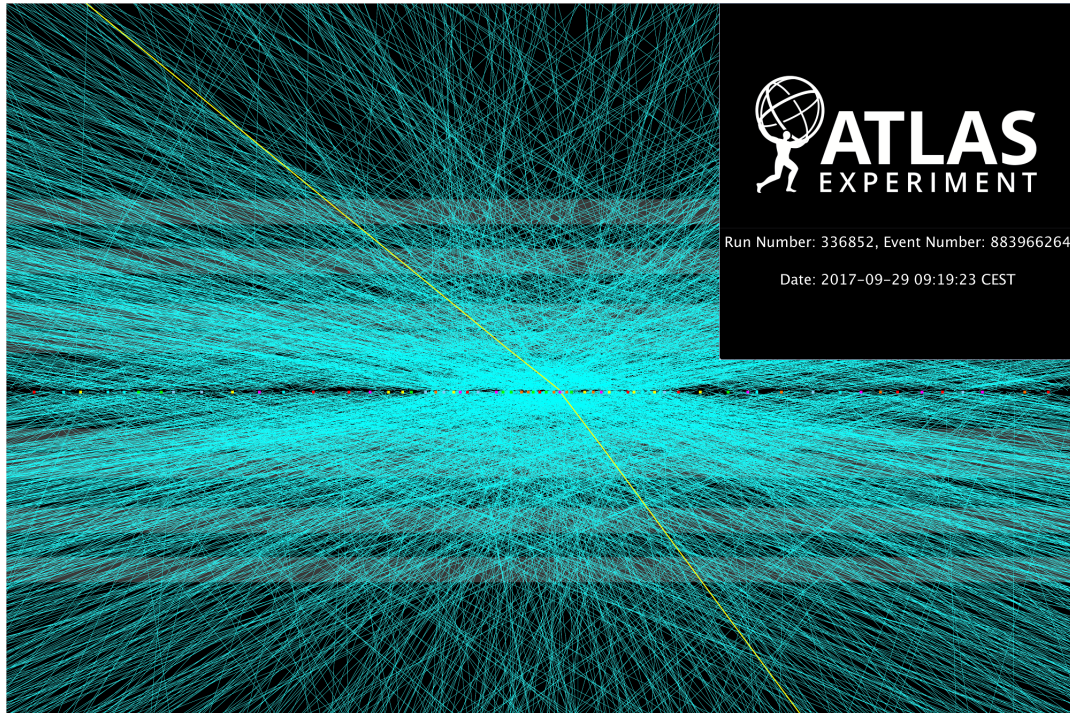
Figure 1.3: An event with a pile-up of 66 as measured and reconstructed at ATLAS on the 29th of September 2017 (Run 336852, Event 883966264). The offset between the single collisions (i.e. the colored spots in the center line) is clearly visible [13].
