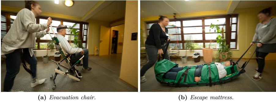
Figure 5.2: Use of the (a) evacuation chair and the (b) escape mattress as assistive devices in the 10MWT. While the wheelchair was always pushed by the assistant, the escape mattress was often pulled backwards to overcome the frictional force more easily. Source: Ralf Eisenbach.
