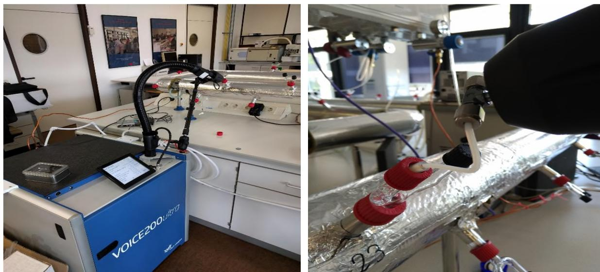
Figure 21: SIFT-MS Setup at the IFA, left: connection to the facility enlarged.
