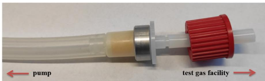
Figure 24: Connection of the aldehyde collection phase Waters Sep-Pak XPoSure to the test gas facility
