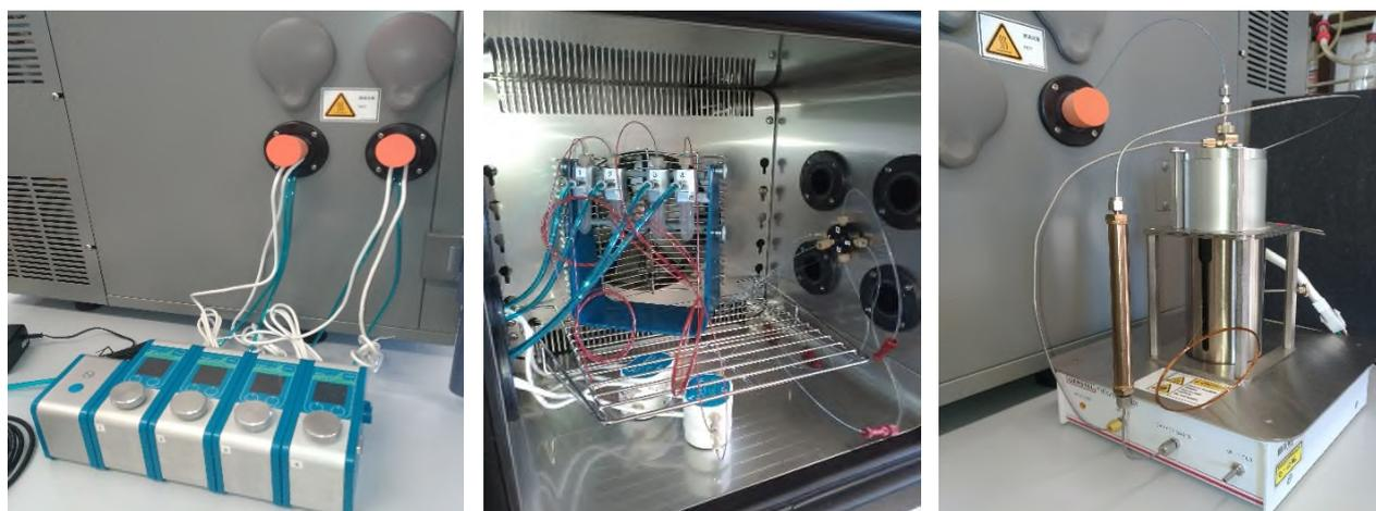
Figure 18: Pressure based dosage system for substances with low vapor pressure. Left: flow controller for pressure-based fluid control (FlowEZ™), middle: climate chamber with substance reservoirs and flow units inside, right: stand-alone Programmed Temperature Vaporizer
