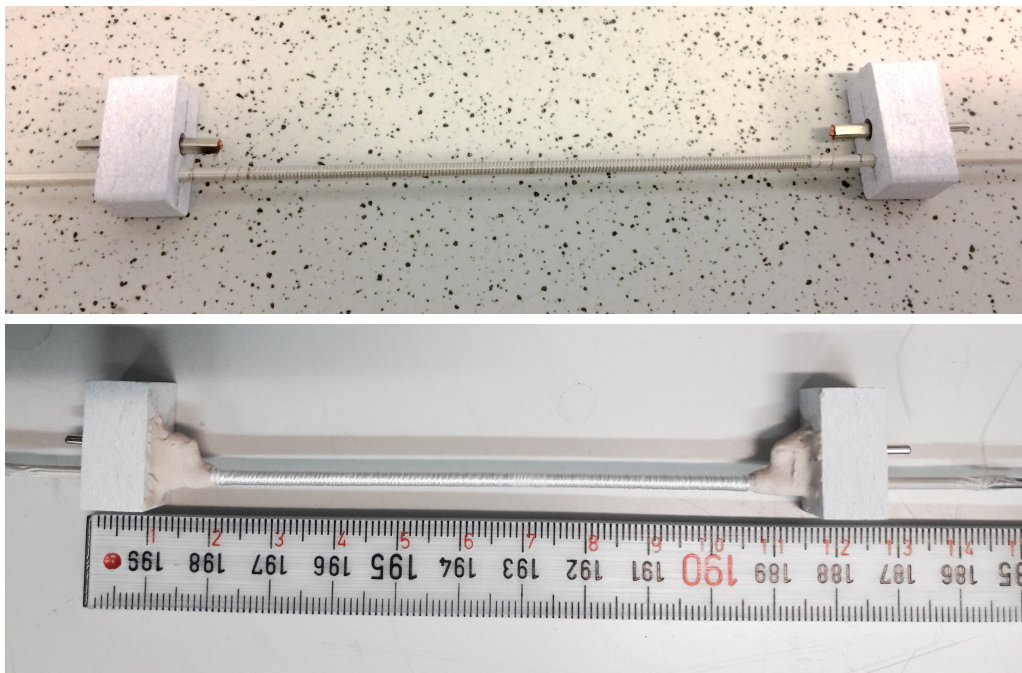
Figure 2.3: Pictures of a self built preconcentration trap in different phases of building. A view on the heating wire/temperature sensor (upper picture) and a view on the glass fiber cord insulated preconcentration trap and fixed plugs with ceramic glue on DoTherm blocks (lower picture).
