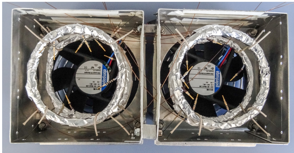
Figure 2.8: Mounting of a full set of four self built LTM columns inside a housing for controlled temperature regulation. Insulated wires hold each column almost contact free in the wind tunnel. One fan cools one pair of columns. The housing also protects the columns from temperature disturbing outside air movements.
