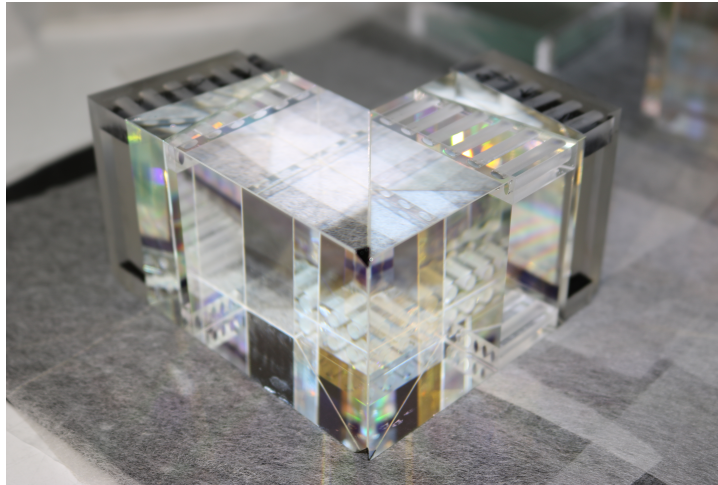
Figure 5.5: Monolithic DASH interferometer. Each spacer, including spacer 1, spacer 2 and parallel spacers, consists of two identical prisms with several through holes.
