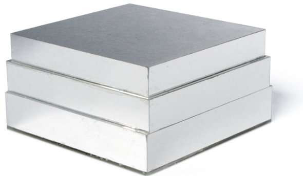
FIGURE 3.3: A crystal block prototype, consisting of 24 \times 24 crystals in the bottom layer. The whole block is covered with a specular reflector, and a lightguide is glued to the bottom crystal array.
