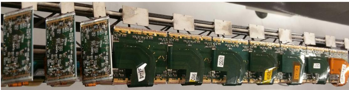
Figure 6.3: Electrical system test setup with inclined dual and flat quad modules [114].
