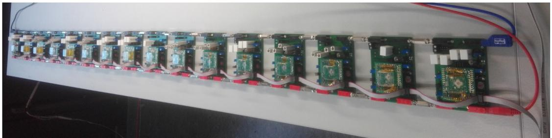
Figure 5.15: Test serial power chain with 16 PSPPv3 chips. The ribbon cable holds the SCB signal lines and goes to the FPGA (not in the picture).
