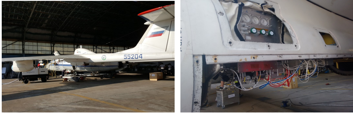
(a) Geophysica M55 in the hangar in Kalamata Airport (KLX) during the test campaign 2016. (b) FunMass mounted in the left wingpod of the aircraft.
