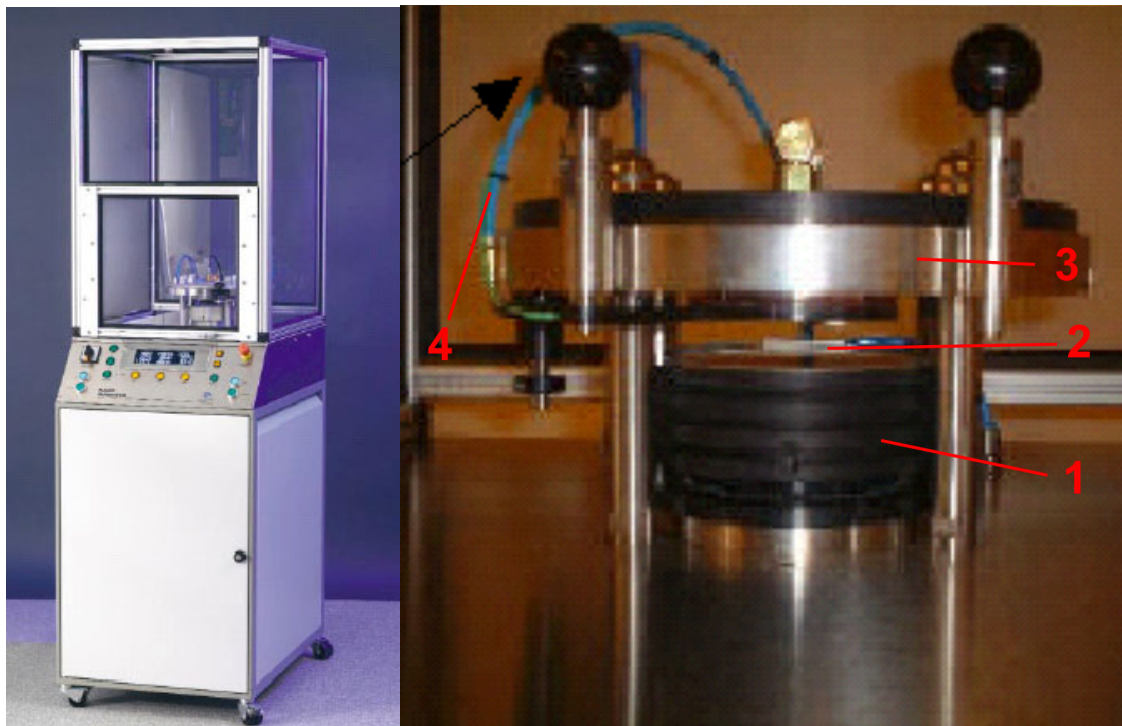
Fig.3-2. Obducat 2.5'' Nanoimprinter. (1– base-plate with heater, 2- space, where the stamp and the sample are placed, one on the other, during printing, 3- upper part with gas volume and membrane, 4- hose with cooling air).
