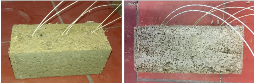
Figure 54: Prisms with thermo-wires. Casted out (left), hardened (right)
