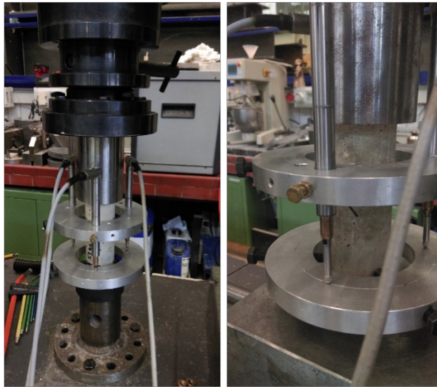
Figure 60a: Configuration of type WAT deformation measuring device
