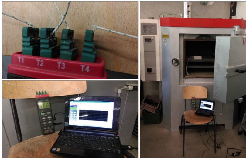
Figure 85: Temperature measurement in tempering oven (Vötsch, type VAW 60/60) for temperatures up to 600°C via a 4-measuring-channel thermo-logger (VOLCRAFT K 204 data logger)
