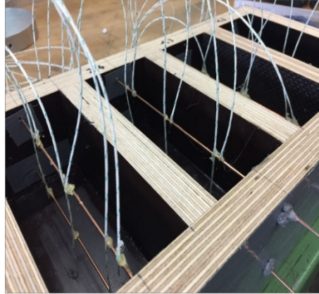
Figure 53: Wooden moulds with two fixed copper rods and fixed thermal wires at different measurement points
