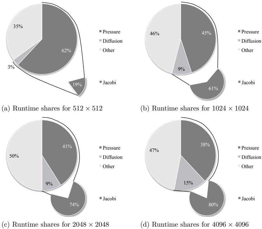
Figure 5.3: JuROR’s runtime shares for fractional steps for various grid resolutions (complete circle: shares of total runtime, adjacent section: share of pressure and diffusion runtime)
