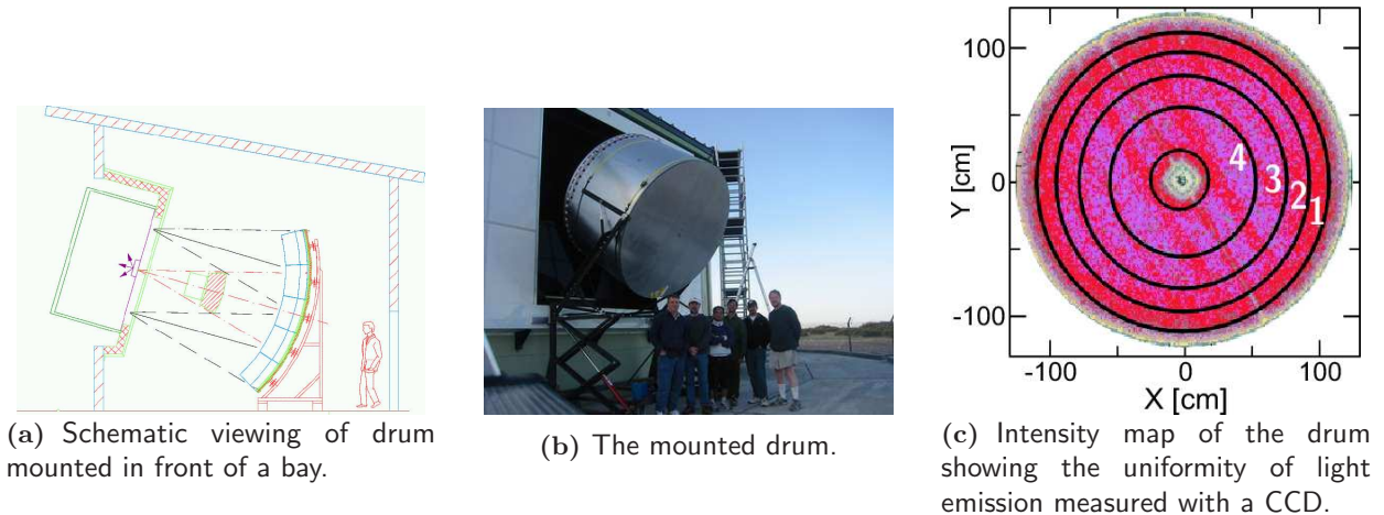
Figure 3.7: Drum calibration, figures taken from [24].
