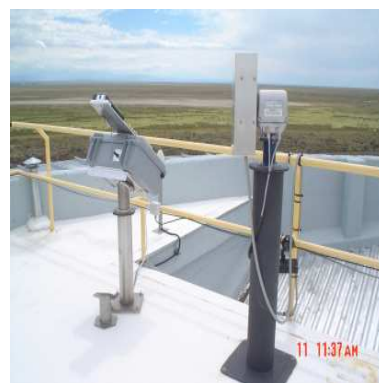
(c) Star monitor (left) mounted on the roof of Los Leones, right beside the cloud camera.
