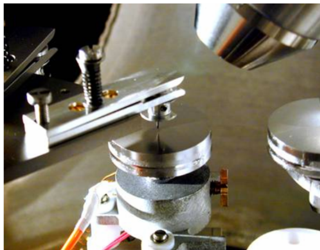
Fig. 2: Inner view of FESM, showing a mirror like Nb sample of 28 mm diameter below a tungsten tip anode ( \sim 1 \mu\text{m} apex radius).
