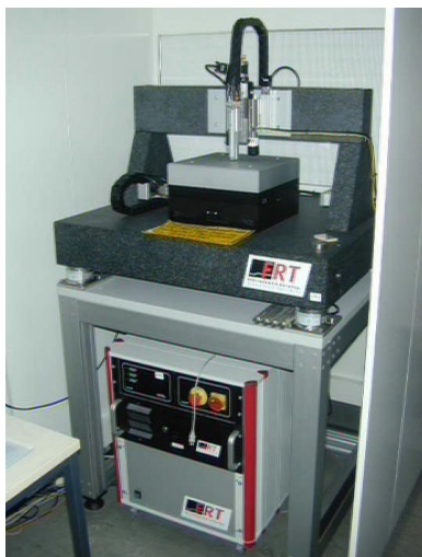
Fig. 3.19. Profilometer with 2 optical sensors and AFM. The granite plate provides stability for the investigations at the nm scale.
