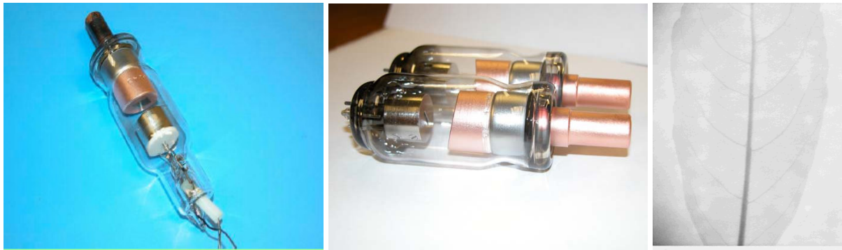
Fig. 5.8. Image of x-ray tubes based on CNT cold cathodes [34] and an x-ray image taken with this tubes.
