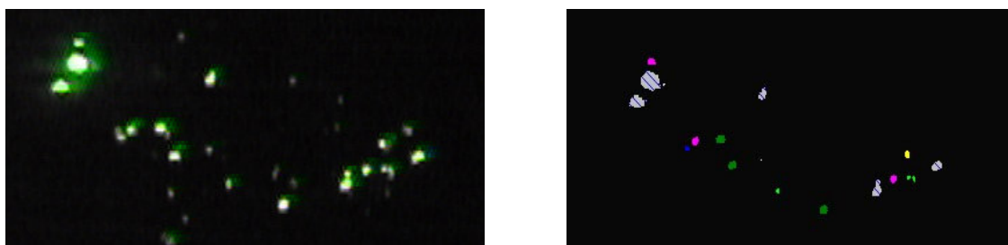
Fig. 3.6. Example of the IMLS luminescent screen image (left) (horizontal size 5 mm) and example of the image analysis with identification of emitters with size above 20 pixels, resulting in 16 clusters and their classification by area.
