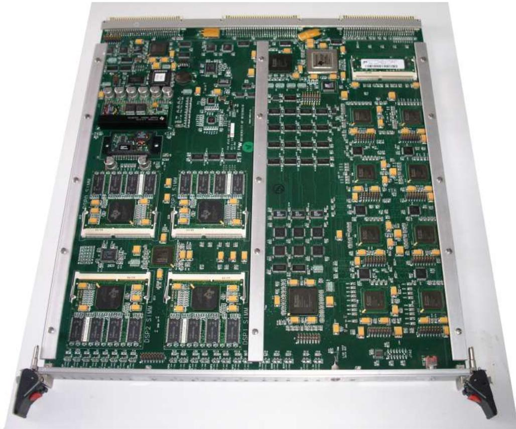
Figure 3.23: Readout Driver (ROD) for the pixel detector.
