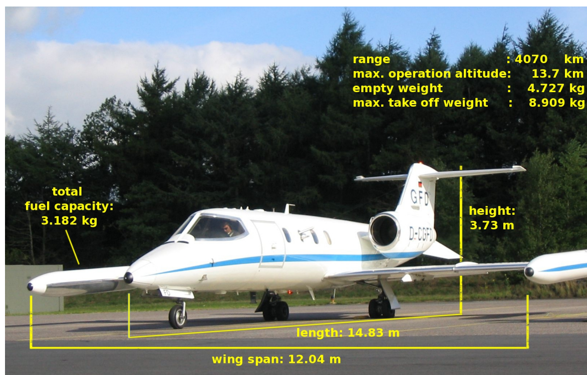
Figure 2.1.: Aircraft used to perform the SPURT campaigns: Learjet 35A D-CGFD, provided by GFD (Hohn, Germany) in co-operation with the company enviscope GmbH (Frankfurt/Main, Germany). Some technical data are drawn in the photograph. Further information can be found under the uniform resource locator address http://www.enviscope.de/home_campaign.html . (Photo by M. Krebsbach)
