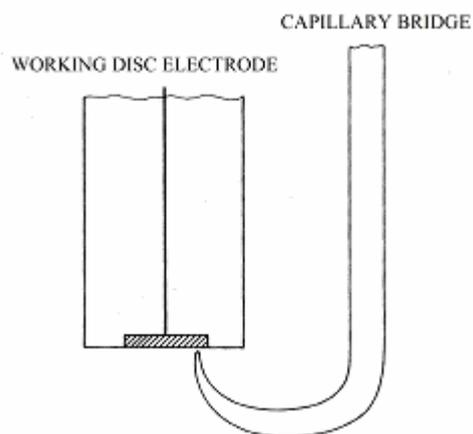
Fig. 7 Disc electrode with capillary bridge.
