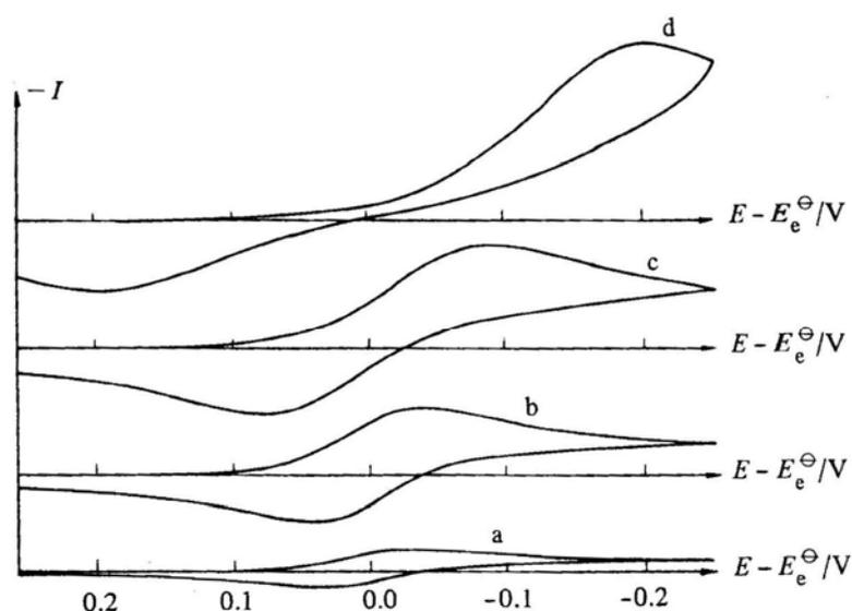
Fig. 6 Irreversible system and its dependence from the scan rate.
