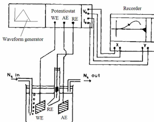
Fig. 1 A schema of the cell used for CVA
