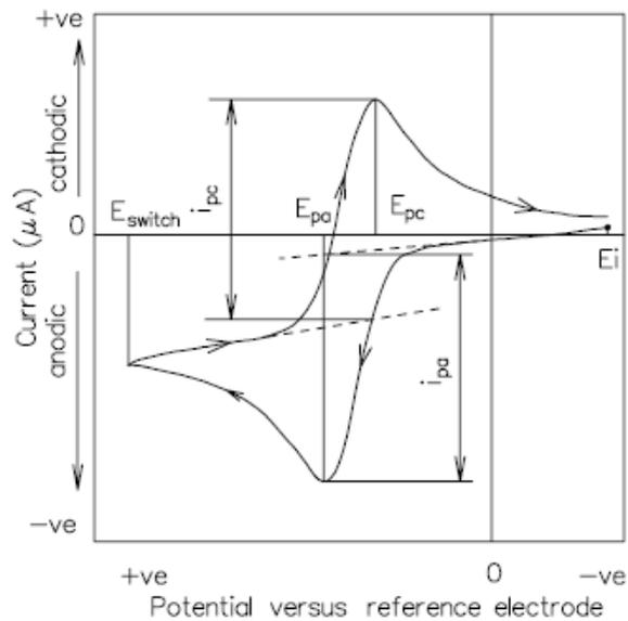
Fig. 4 Basic parameters for the cyclic voltammetry:
