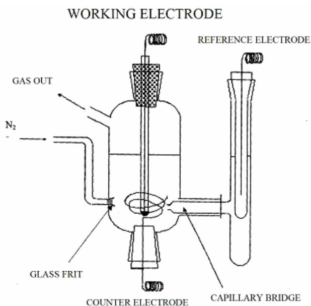
Fig. 8 Typical electrochemical cell
