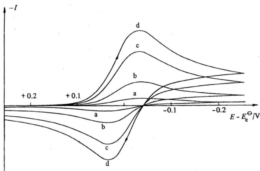
Fig. 5 Reversible system and its dependence from the scan rate.
