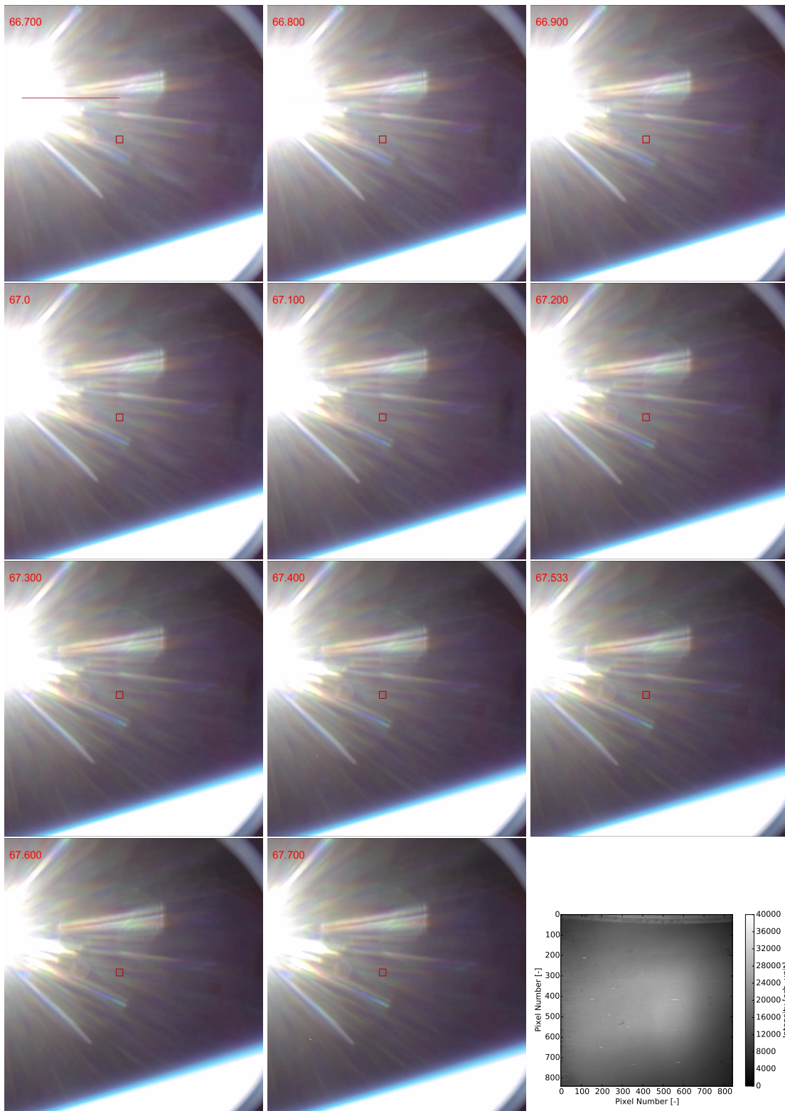
Figure D.1.: Series of VisCAM images after YoYo-despin and before rocket separation anomaly with the corresponding interferogram. The time stamp in the left upper corner of each image shows the time after lift-off in [s].
