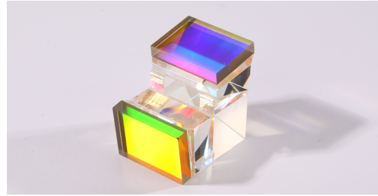
(b) Assembled SHS for the precursor mission.
