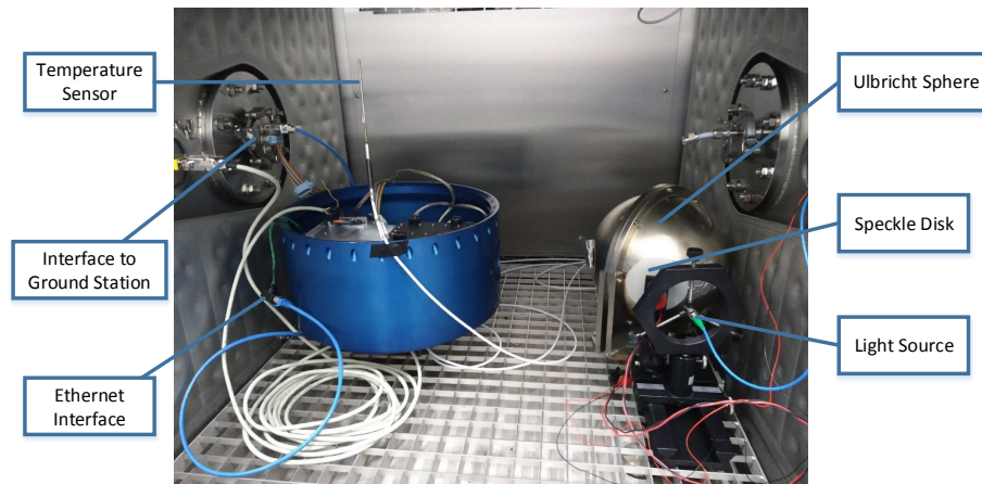
Figure 7.6.: Setup for the T-Vac tests of the instrument at the Research Centre Jülich.
