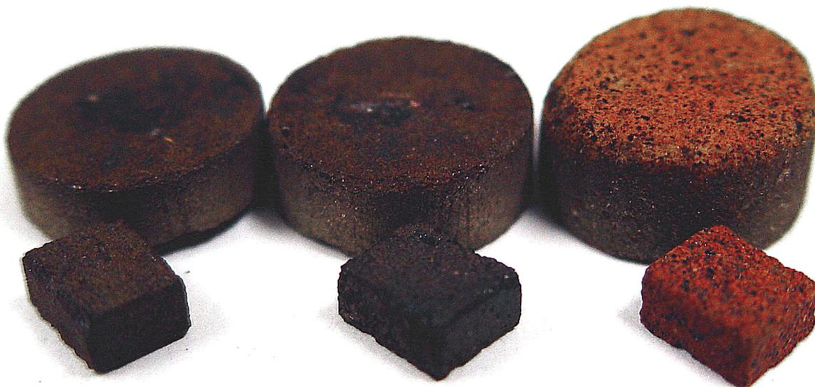
Abbildung 107: Kraft-Lignin-Phenoplaste (links: Kraft-Lignin-Phenol-Phenoplast; Mitte: Kraft-Lignin-4-Ethylphenol-Phenoplast; rechts: Kraft-Lignin-Resorcin-Phenoplast)
