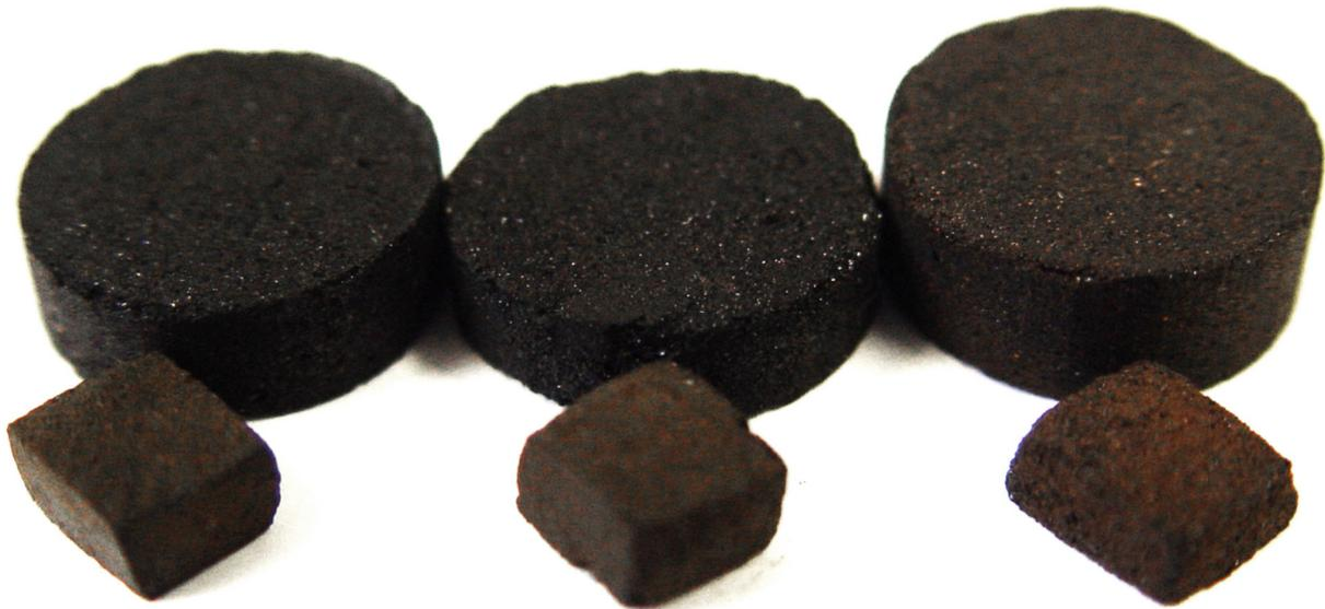
Abbildung 112: Organosolv-Lignin-Phenoplaste (links: Organosolv-Lignin-Phenol-Phenoplast; Mitte: Organosolv-Lignin-4-Ethylphenol-Phenoplast; rechts: Organosolv-Lignin-Resorcin-Phenoplast)
