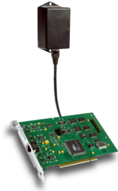
Figure 6.5: Boltek StormTracker PCI Card with antenna. From [129].
