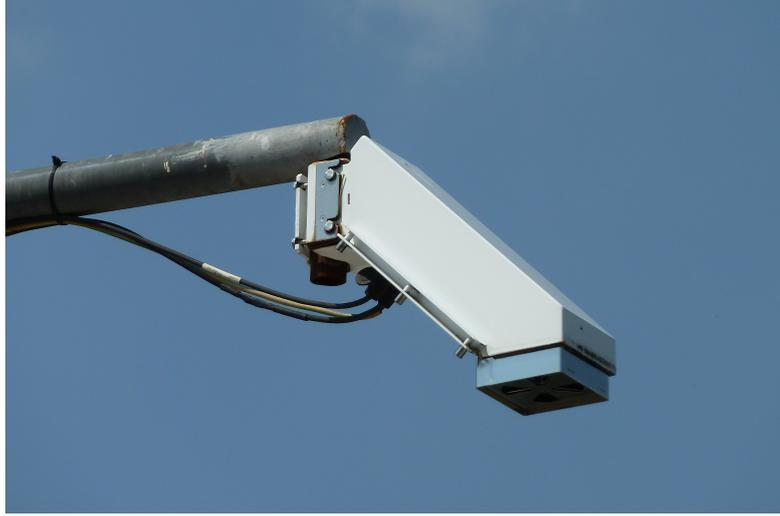
Figure 6.1: Mounted CS110 E-field mill in Karlsruhe
