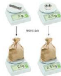
Picture 1: If you know the mass of one piece you can calculate the number of pieces in the bag when you weigh it, e.g. how many pieces are in a bag that weighs 10 kg?
