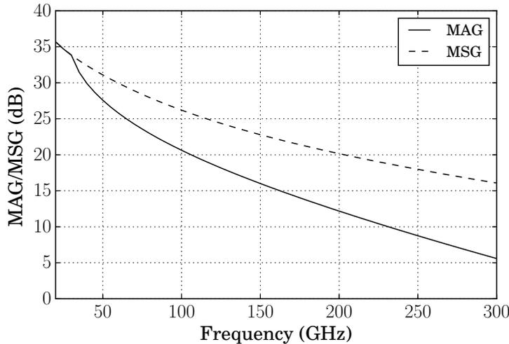
Figure 3.1: Simulated MAG for a single-ended cascode stage is 9.4 dB at 240 GHz. The HBTs are biased at the peak  $f_{max}$  current of 12.5 mA, and transistors with an emitter area of  $8 \times (0.96 \times 0.12) \mu m^2$  are used.
