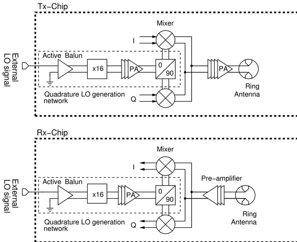
Figure 4.1: Block-diagram of the 240 GHz fully-integrated direct-conversion quadrature Tx and Rx chipset with wideband on-chip antennas. The IF inputs of the Tx and Rx are terminated with on-chip  $50\ \Omega$  resistances for wideband IF matching [11].
