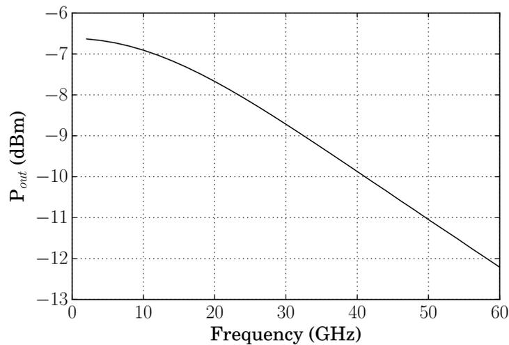
Figure 3.51: Simulation results for the IF bandwidth characterization of the 240 GHz up-conversion mixer. The 3-dB IF bandwidth is 38 GHz.
