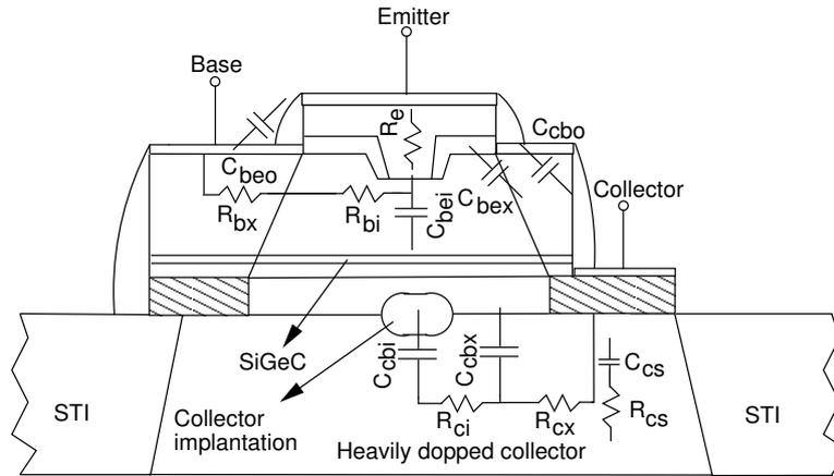
Figure 2.5: Layout cross-section of a SiGe HBT from IHP Microelectronics based on the double-polysilicon self-aligned (DPSA) architecture [131] with a lateral intrinsic-to-extrinsic base link.
