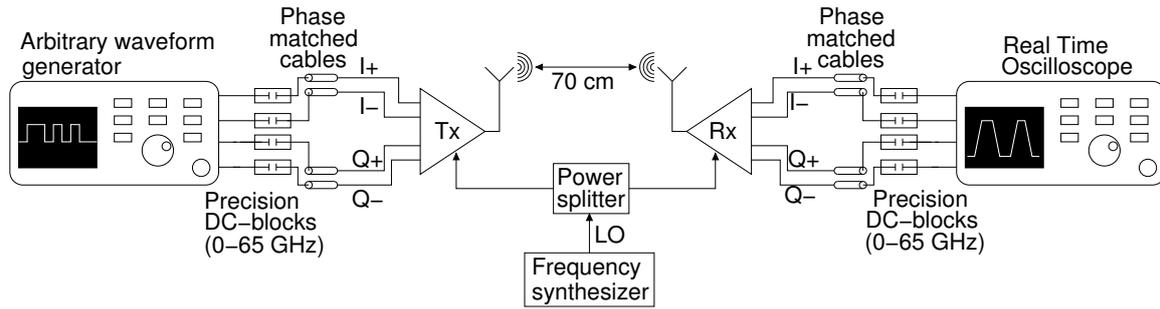
Figure 4.22: Measurement setup for the 240 GHz high data-rate communication system for a wireless link of 70 cm. An AWG is used to feed the Tx IF input with PRBS9 data, and the IF outputs of the Rx are connected to a real-time oscilloscope.
