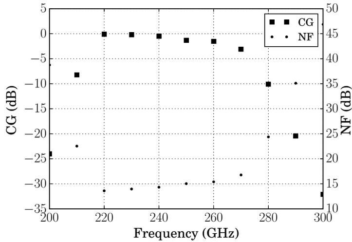
Figure 3.55: Simulation results for the RF bandwidth characterization of the 240 GHz down-conversion mixer. The 3-dB RF bandwidth is 52 GHz. At 240 GHz, CG is -0.5 dB and NF is 14.2 dB.
