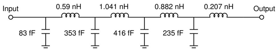
Figure 4.2: Schematic of the 8<sup>th</sup> order low-pass LC filter from the 1<sup>st</sup> design iteration. The filter is synthesized using the design methodology presented in [113, 142].
