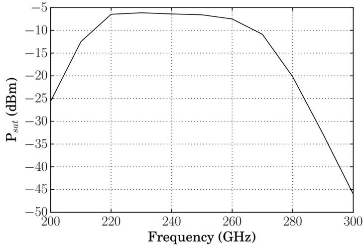
Figure 3.52: Simulation results for the RF bandwidth characterization of the 240 GHz up-conversion mixer. The 3-dB large-signal RF bandwidth is 50 GHz.
