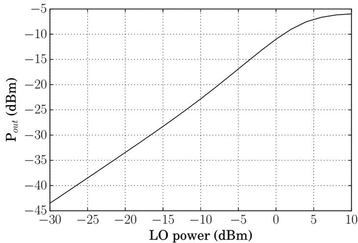
Figure 3.53: Simulation results for the variation of  $P_{out}$  with LO power for the 240 GHz up-conversion mixer. For stronger switching, an LO power of 5 dBm and higher is required at the input of the  $90^\circ$  coupler.
