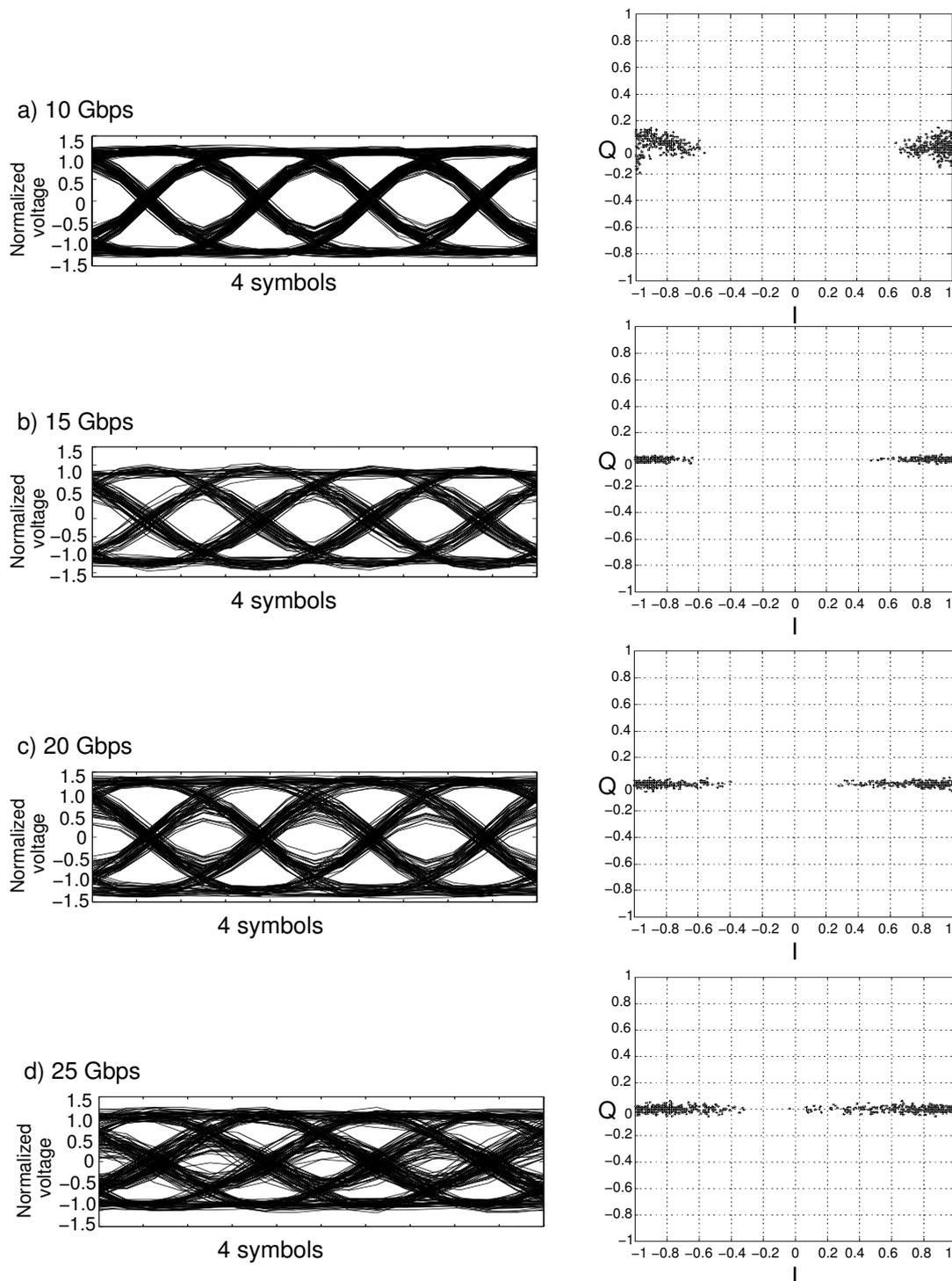
Figure 4.23: Eye-diagram and constellation for BPSK modulation scheme at a carrier frequency of 240 GHz. The measured rms EVM is a) 16% at 10 Gbps, b) 17.8% at 15 Gbps, c) 24% at 20 Gbps and d) 30% at 25 Gbps.
