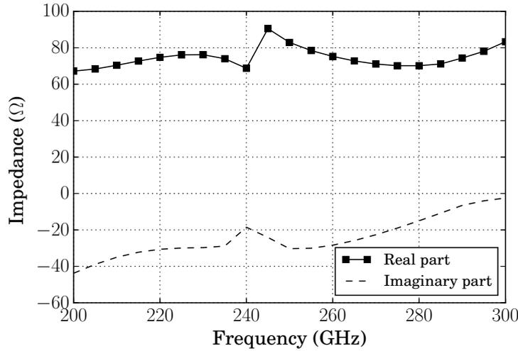
Figure 4.20: Simulated differential input impedance for a  $50\ \Omega$  load termination at the single-ended output of the Marchand-balun. From 200-300 GHz, the input impedance is complex and the real part varies from 75-80  $\Omega$ .
