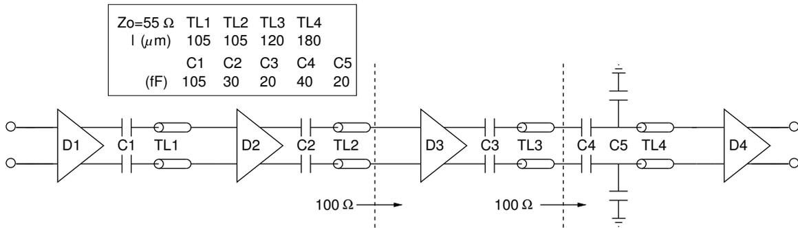
Figure 3.37: Interstage matching network of the 240 GHz LO signal source. The inputs of D3 and D4 are matched to a differential  $100\ \Omega$  impedance. The doubler D4 is connected to a three-stage 240 GHz PA with  $50\ \Omega$  lines, and is not shown here.
