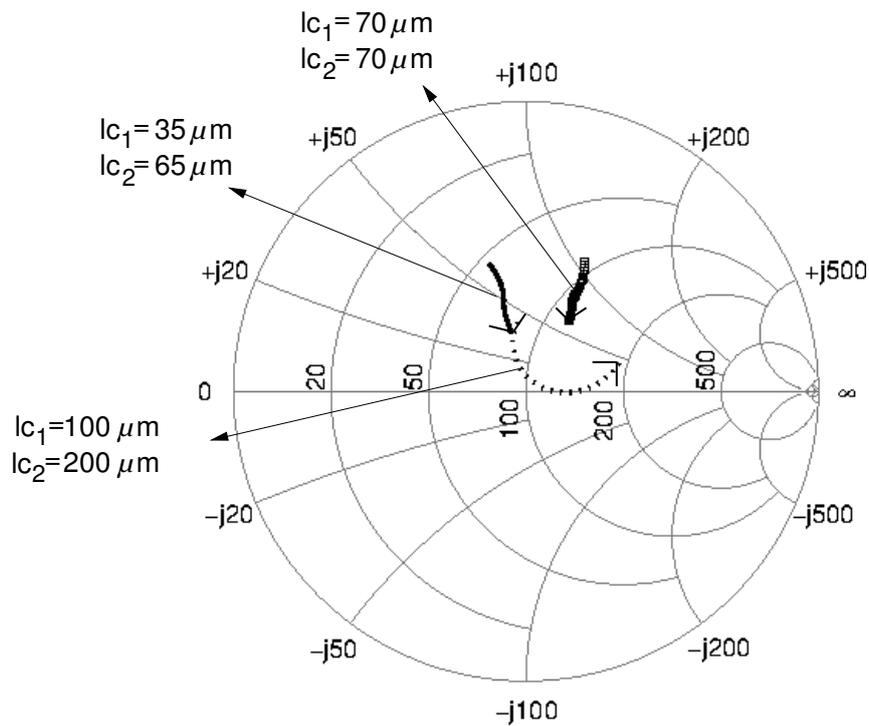
Figure 3.22: Simulated  $Z_d$  at the 4:1 power-combiner input from 200-240 GHz for three line dimensions: a)  $lc_1=35 \mu\text{m}$ ,  $lc_2=65 \mu\text{m}$ . b)  $lc_1=lc_2=70 \mu\text{m}$ . c)  $lc_1=100 \mu\text{m}$ ,  $lc_2=200 \mu\text{m}$ .
