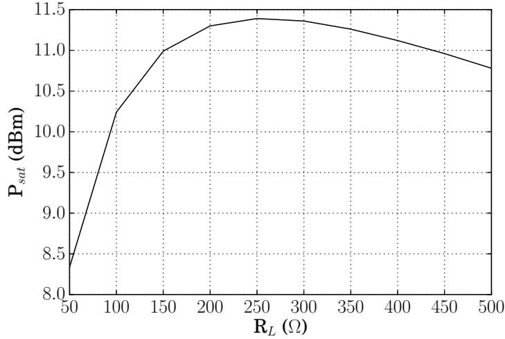
Figure 3.5: Simulated  $P_{sat}$  at 240 GHz for different  $R_L$ . The optimum impedance at the collector of the output stage is 320  $\Omega$ , and the corresponding  $P_{sat}$  is 11.3 dBm. The  $P_{sat}$  is reduced only to 10.2 dBm for  $R_L=100 \Omega$ .
