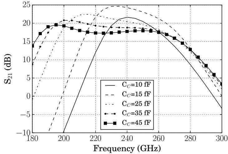
Figure 3.9: Simulated small-signal gain variation of the 240 GHz PA for different  $C_c$ . The bandwidth and gain-ripple increases with  $C_c$ . For  $C_c = 15$  fF, the simulated peak gain is 25 dB and the 3-dB bandwidth is 40 GHz.
