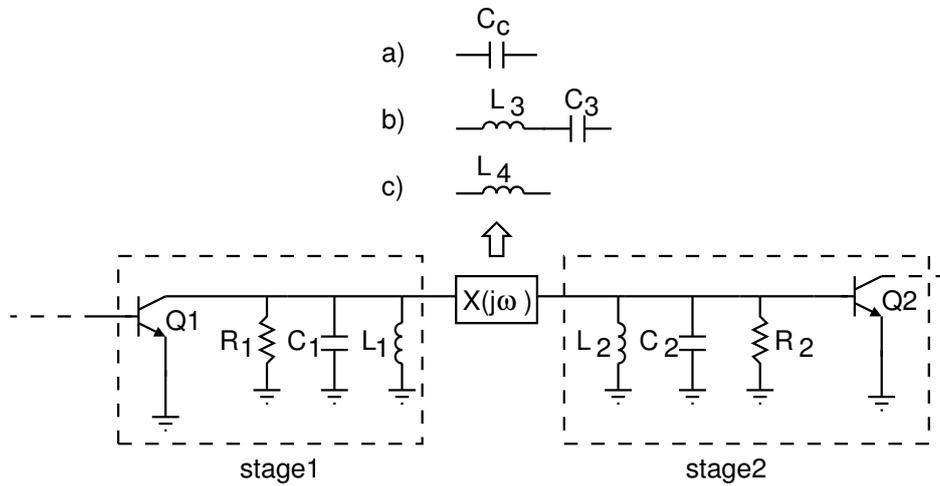
Figure 2.2: Schematic of a two-stage tuned CE amplifier. A passive network  $X(j\omega)$  isolates the capacitors  $C_1$  and  $C_2$ . The network  $X(j\omega)$  can be implemented using a) a series-capacitor  $C_c$ , b) a series-LC circuit  $L_3, C_3$ , and c) a series-inductor  $L_4$ .
