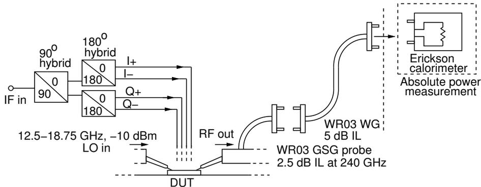
Figure 4.10: Measurement setup for the on-wafer characterization of the 240 GHz Tx. A GSG probe (DC-40 GHz) with a 2.9 mm K-connector is used to couple the external LO signal to the chip. A WR03 GSG probe is used at the Tx output.
