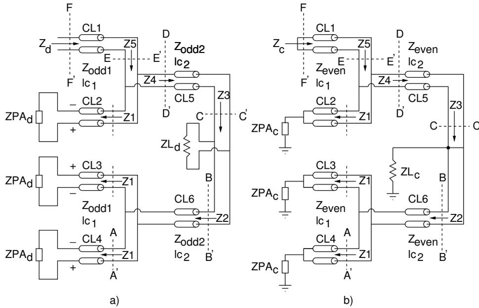
Figure 3.20: Impedance transformation at the 4:1 power-combiner input taking into account the loading effect of the unit PAs. a) The differential input impedance is  $Z_d$ . b) The common-mode input impedance is  $Z_c$ . Here,  $ZPA_d$  and  $ZPA_c$  are the respective large-signal differential and common-mode output impedances of the unit PAs.
