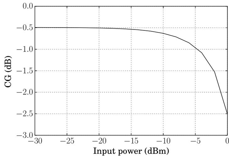
Figure 3.58: Simulation results for  $IP_{1dB}$  of the 240 GHz down-conversion mixer. At 240 GHz,  $IP_{1dB}$  is -2.5 dBm. For this simulation, a LO drive power of 5 dBm is used.
