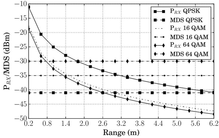
Figure 4.21: Simulated maximum range for a high data-rate communication system using the 240 GHz packaged-Tx and Rx chipset for different modulation schemes. For a BER of  $10^{-6}$ , the maximum estimated range for QPSK modulation is 6.2 m, for 16-QAM it is 1.4 m, and for 64-QAM it is 0.8 m.
