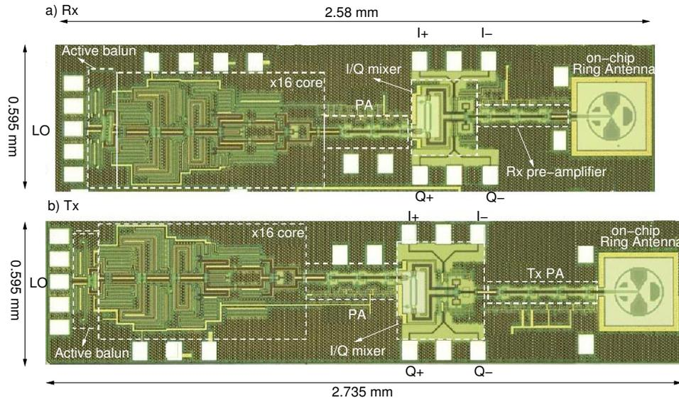
Figure 4.9: Chip-micrograph of the 240 GHz fully-integrated quadrature Tx and Rx with on-chip antennas. The chip area including the pads is a)  $1.535 \text{ mm}^2$  for the Rx, and b)  $1.627 \text{ mm}^2$  for the Tx.
