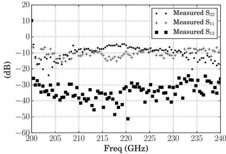
Figure 3.31: From 200-240 GHz, the measured  $S_{11} \leq -10$  dB and  $S_{12} \leq -30$  dB for the 200-225 GHz combiner-PA.
