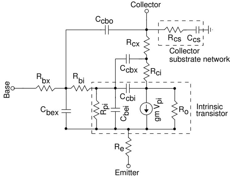
Figure 2.6: Small-signal lumped equivalent circuit for the device shown in Figure 2.5 with the various parasitic elements [130, 131].
