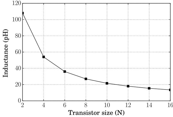
Figure 3.4: Tuning inductance versus transistor size at 240 GHz for a single-ended cascode stage. The emitter area of the transistor is  $N \times (0.96 \times 0.12) \mu\text{m}^2$ . The required tuning inductance at 240 GHz is 28 pH for  $N=8$ .
