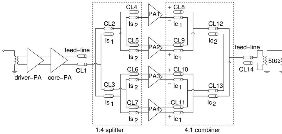
Figure 3.19: Block diagram of the 200-225 GHz combiner-PA [146]. The output power from the core-PA is split using a 1:4 power-splitter (CL2-CL7). A 4:1 coupled microstrip-line based ZDC (CL8-CL13) combines the output from the unit PAs (PA1-PA4).
