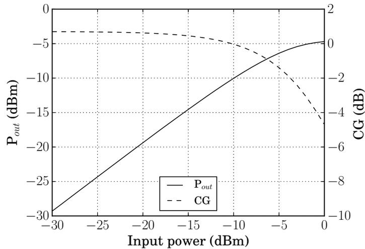
Figure 3.50: Simulation results from the linearity characterization of the 240 GHz up-conversion mixer. The peak CG is 0.7 dB,  $P_{sat}$  is -5 dBm and  $OP_{1dB}$  is -8 dBm. A 25 MHz IF signal (-5 dBm) is used for this simulation.
