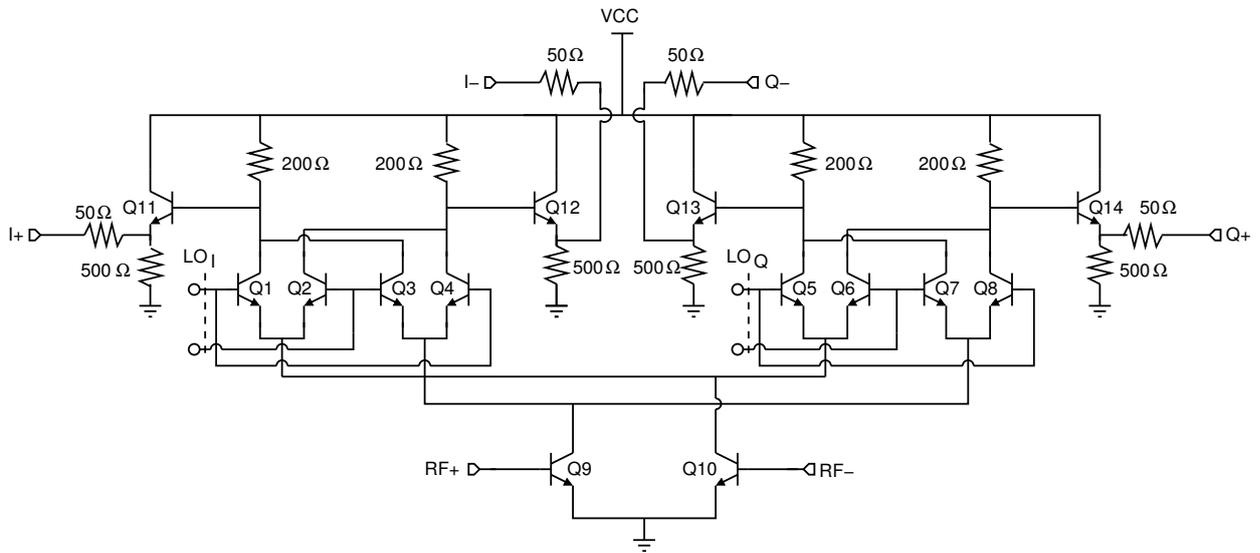
Figure 3.54: Schematic of the 240 GHz quadrature down-conversion mixer. The transconductance stage (Q9-Q10) injects the RF current into the switching quads of the I-mixer (Q1-Q4) and Q-mixer (Q5-Q8). The optimum load impedance is 200  $\Omega$ .
