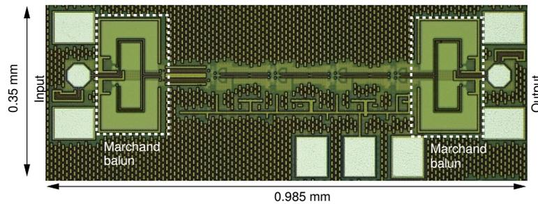
Figure 3.12: Chip-micrograph of the 240 GHz PA. The total chip area including the auxiliary Marchand-baluns and pads is 0.345 mm<sup>2</sup>.
