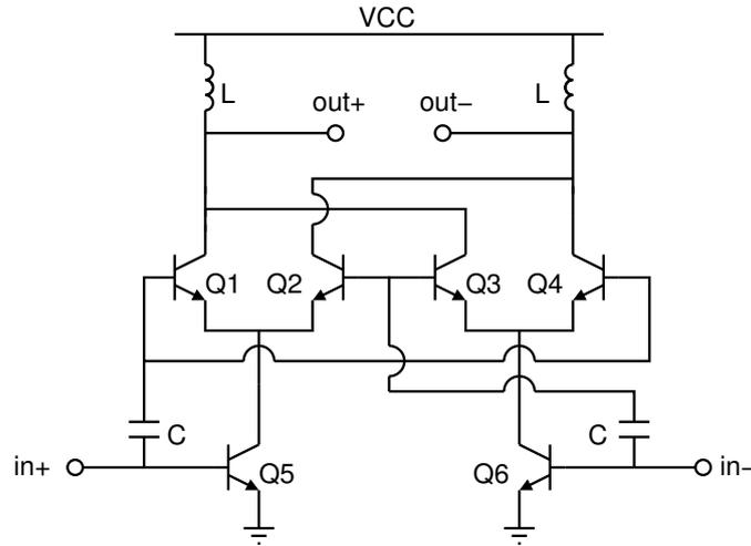
Figure 2.1: Schematic of a frequency doubler circuit based on the Gilbert-cell topology. The RF and LO signal inputs are ac-coupled, and self-multiplication results in the generation of a dc-offset and a  $2^{nd}$  harmonic component.
