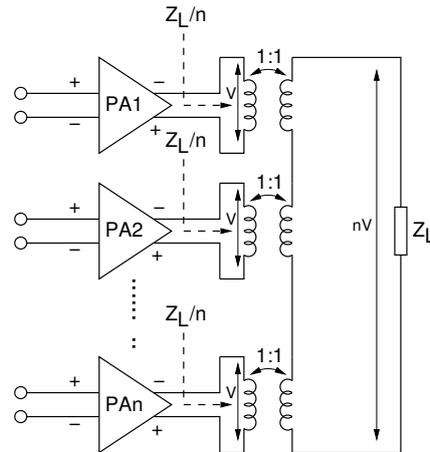
Figure 2.8: Transformer-based series power-combiner. In this topology, the output voltages from the unit PAs are summed at the combiner output. At the output of the unit PAs, the load impedance  $Z_L$  is transformed to  $Z_L/n$ .
