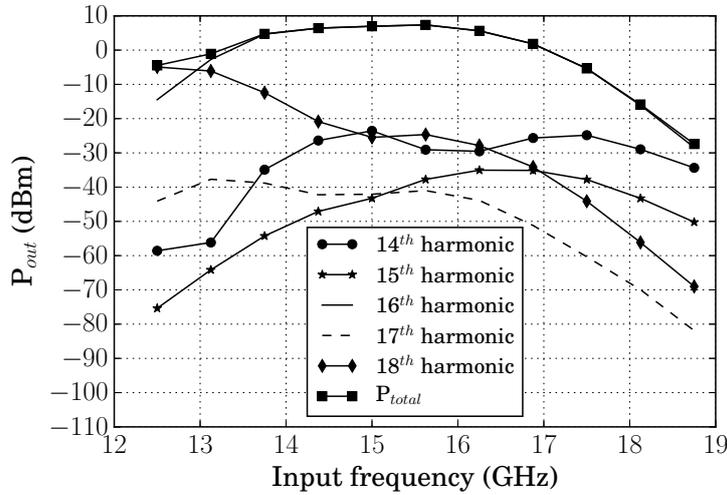
Figure 3.40: Simulated  $P_{out}$  at the different harmonics for an input LO power of -10 dBm. At 15 GHz,  $P_{out}$  at the 16<sup>th</sup> harmonic is 7.3 dBm. The relative attenuation of the 14<sup>th</sup>, 15<sup>th</sup> and 17<sup>th</sup> harmonic is at least 25 dB. The effect of the 18<sup>th</sup> harmonic only starts at input frequency less than 13.25 GHz, and hence can be ignored.
