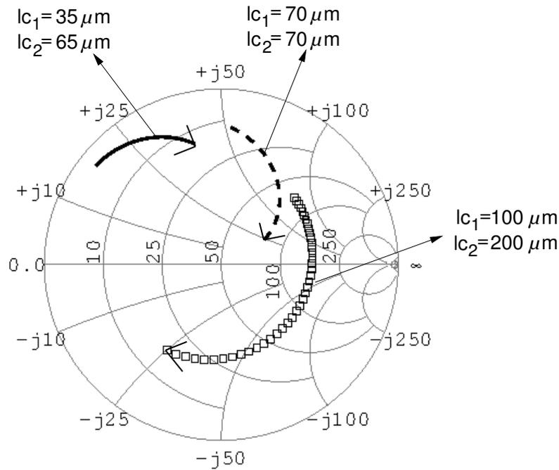
Figure 3.23: Simulated  $Z_c$  at the 4:1 power-combiner input from 200-240 GHz for three line dimensions: a)  $lc_1=35 \mu\text{m}$ ,  $lc_2=65 \mu\text{m}$ . b)  $lc_1=lc_2=70 \mu\text{m}$ . c)  $lc_1=100 \mu\text{m}$ ,  $lc_2=200 \mu\text{m}$ .
