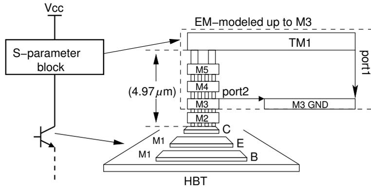
Figure 3.3: EM modeling of the parasitic via-inductance in HFSS, port1 is defined as a wave-port and port2 is defined as a lumped-port. The ground plane is in the M3 metal layer.
