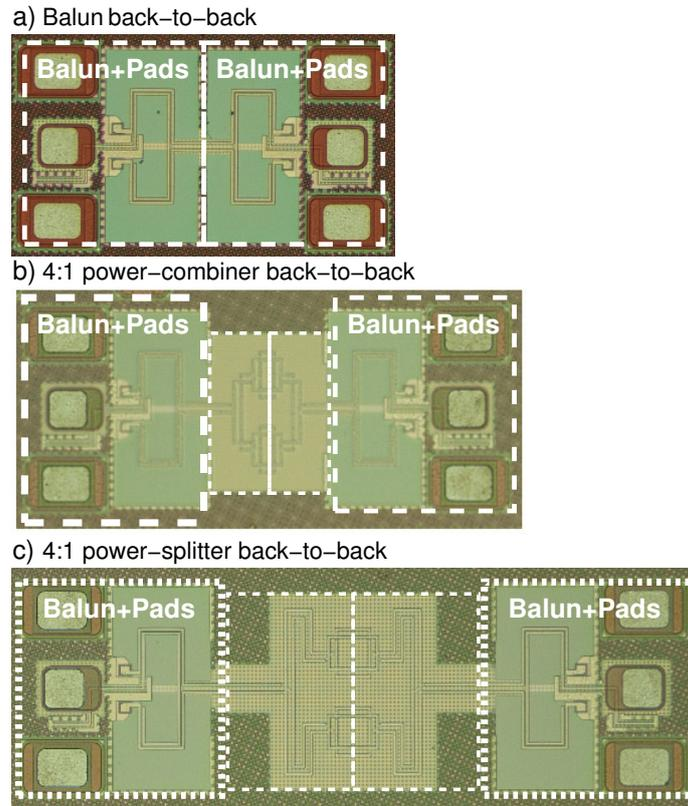
Figure 3.26: Chip-micrograph of the additional breakout structures for estimating the insertion loss of the 1:4 power-splitter and 4:1 power-combiner. a) Back-to-back Marchand-baluns. b) Back-to-back 4:1 power-combiner with Marchand-baluns. c) Back-to-back 1:4 power-splitter with Marchand-baluns.
