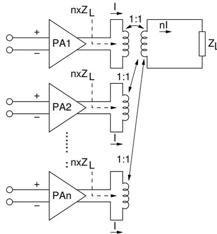
Figure 2.9: Transformer-based parallel power-combiner. In this topology, the output current from the unit PAs are added at the output of the combiner. At the output of the unit PAs, the load impedance  $Z_L$  is transformed to  $n \times Z_L$ .
