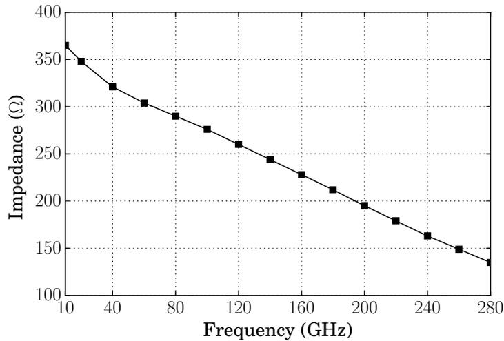
Figure 2.7: Simulated real part of the output impedance of a cascode stage at different resonant frequencies. The output impedance decreases only by 14% from 60 to 120 GHz range while it decreases by 44% from 140 to 280 GHz [23].
