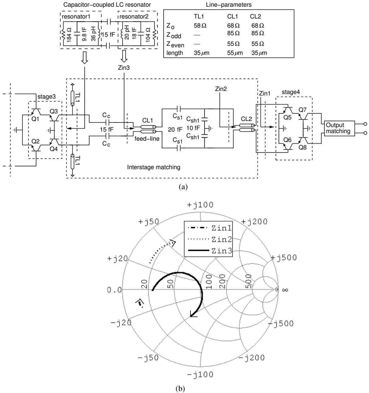
Figure 3.8: a) Wideband interstage matching of the 240 GHz PA based on capacitor-coupled LC resonators. The series capacitor  $C_c$  couples resonator1 and resonator2. b) Impedance transformation from  $Z_{in1}$  (input impedance of stage4) to  $Z_{in3}$  (synthesis of resonator2) from 200-300 GHz.
