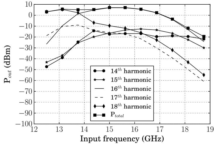
Figure 3.41: Simulated  $P_{out}$  at the different harmonics for an input LO power of 0 dBm. The effect of the spurious 18<sup>th</sup> harmonic increases significantly below 14.25 GHz, and this results in  $P_{total}$  remaining constant. This substantially limits the usable input frequency range. Hence, the optimum input LO power is -10 dBm.
