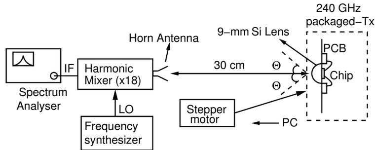
Figure 4.16: Setup for the measurement of the antenna radiation pattern of the 240 GHz packaged-Tx. A 2-D rotational stage controlled by a stepper motor is used for precise alignment. An external WR03 VNA extension module is used as Rx.
