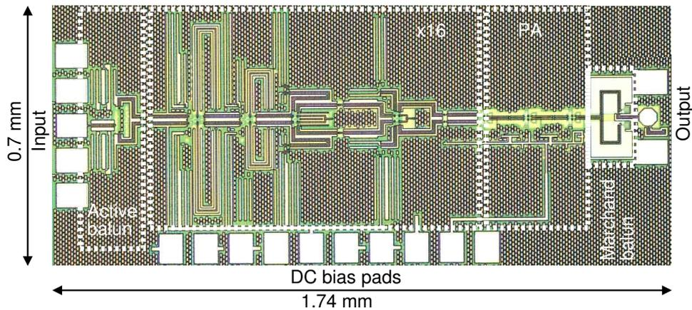
Figure 3.42: Chip-micrograph for the breakout of the 240 GHz LO signal source. The total chip area including the pads is 1.218 mm<sup>2</sup>. For single-ended on-wafer measurements, an auxiliary Marchand-balun has been added at the output [88].
