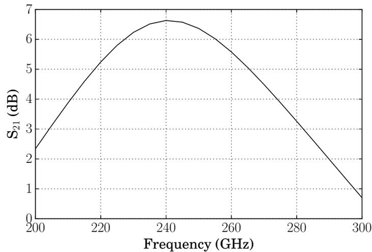
Figure 3.7: Simulated small-signal gain for the full EM simulated model of the output stage of the 240 GHz PA shown in Figure 3.6. The peak gain is 6.5 dB at 240 GHz.
