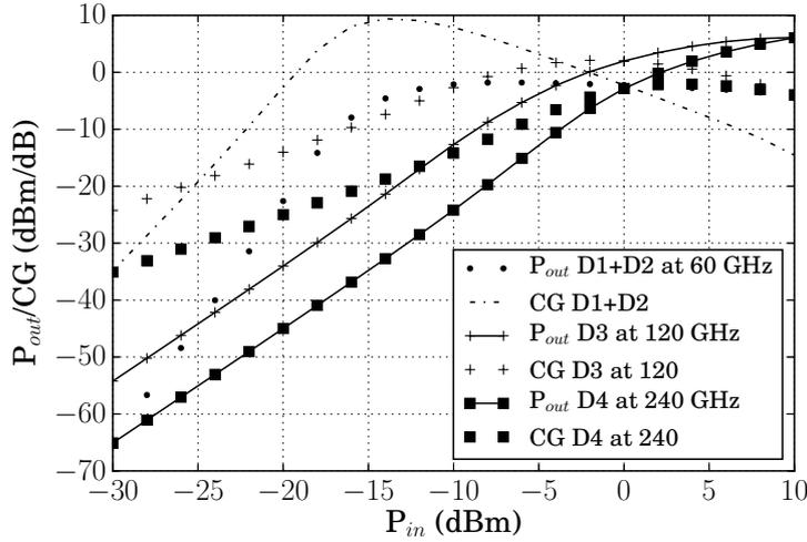
Figure 3.35: Simulated large-signal characteristics for the doublers D1+D2, D3 and D4 for an overall output frequency of 240 GHz. For an output power of -2.8 dBm at 240 GHz, the corresponding LO power at the input of D1 is -10 dBm.
