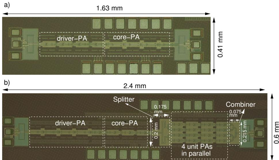
Figure 3.25: Chip-micrograph of the 200-225 GHz a) breakout-PA: The chip area is  $0.67 \text{ mm}^2$ , and b) combiner-PA: The chip area is  $1.44 \text{ mm}^2$ . The unit PAs are identical to the core-PA.
