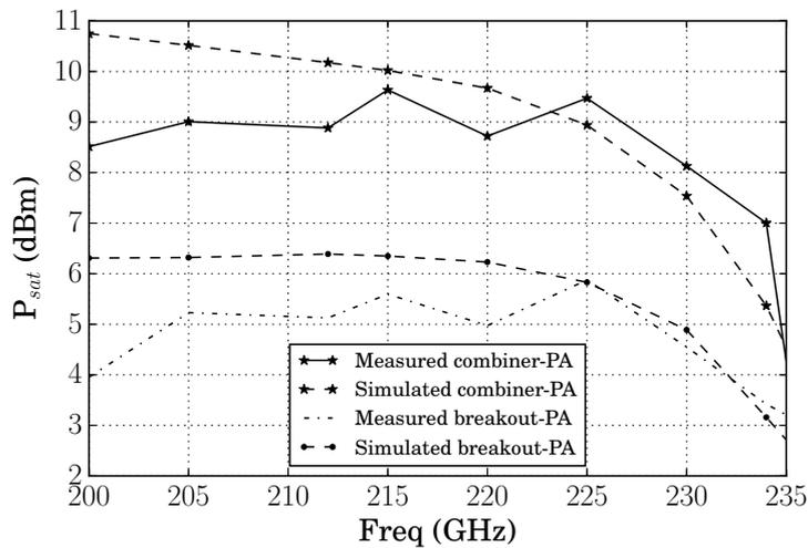
Figure 3.28: Hardware correlation for the large-signal bandwidth characterization of the 200-225 GHz combiner-PA and breakout-PA. The peak  $P_{sat}$  for the combiner-PA is 9.6 dBm at 215 GHz, and the 3-dB large-signal bandwidth is 34 GHz (200-234 GHz).
