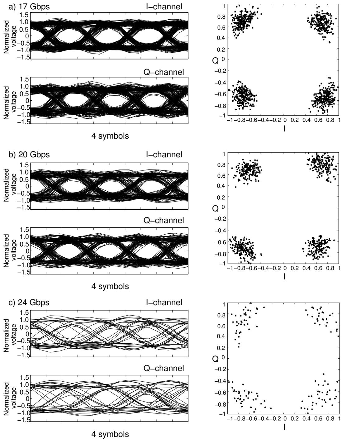
Figure 4.24: Eye-diagram and constellation diagram for QPSK modulation scheme at a carrier frequency of 240 GHz. The measured rms EVM is a) 15.7% at 17 Gbps, b) 17% at 20 Gbps and c) 24% at 24 Gbps.
