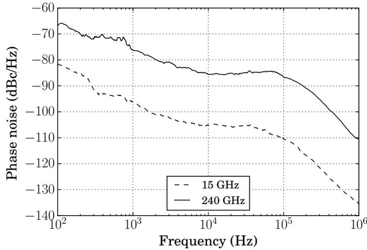
Figure 3.48: Measured phase-noise of the 240 GHz LO signal source. An external 15 GHz signal (-10 dBm) with a phase-noise of -135 dBc/Hz (1 MHz offset) is used. The measured phase-noise at 240 GHz is -110 dBc/Hz, which is a degradation of 25 dB.
