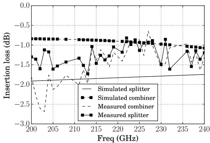
Figure 3.27: Hardware correlation for the insertion-loss of the 1:4 power-splitter and 4:1 power-combiner. From 200-240 GHz, the measured insertion loss is in the 1-2 dB range.
