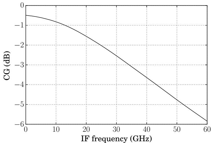
Figure 3.56: Simulation results for the IF bandwidth characterization of the 240 GHz down-conversion mixer. For  $R_c=200 \Omega$ , the peak CG is -0.5 dB and the 3-dB IF bandwidth is 35 GHz. An IF frequency of 33 MHz is used for this simulation.
