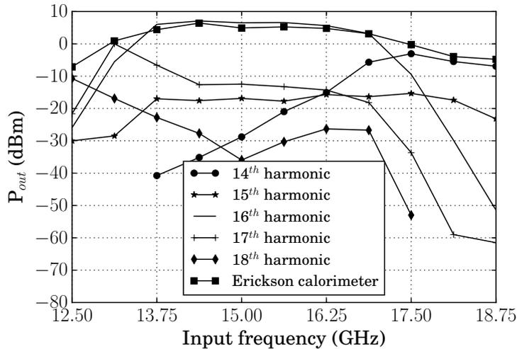
Figure 3.45: Measured  $P_{out}$  at the different harmonics at the output of the 240 GHz LO signal source for an input power of -10 dBm. The output power at the 16<sup>th</sup> harmonic (220–270 GHz) is close to absolute power measurements for input frequencies in the 13.75–16.875 GHz range.
