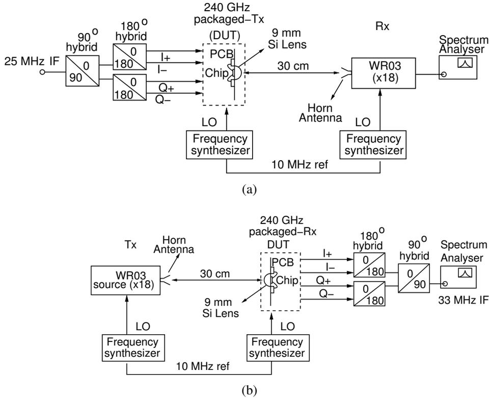
Figure 4.14: Measurement setup for the free-space RF characterization of the 240 GHz Tx and Rx over a 30 cm wireless link. a) Tx: A pre-calibrated WR03 VNA extension module with an external horn-antenna with WR3.4 waveguide interface is used as the Rx. b) Rx: A pre-calibrated WR03 VNA extension module with an external horn-antenna with WR3.4 waveguide interface is used as the Tx.
