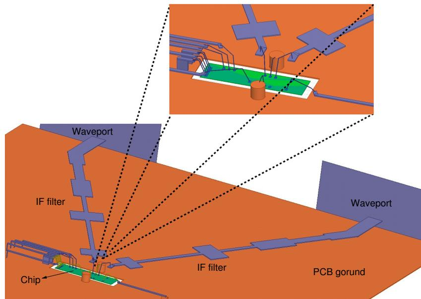
Figure 4.6: 3D model for EM simulation of the PCB filter (including the effect of wire-bond connections) using HFSS. The chip and PCB ground pads are included to accurately model the ground return current.
