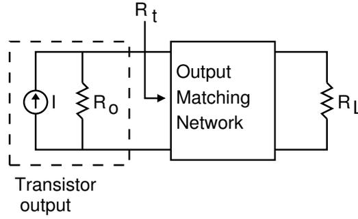
Figure 2.4: Equivalent current source representation of the output stage of a class-A PA. The output matching network transforms the load impedance  $R_L$  to  $R_t$ . Here,  $R_o$  is the real part of the output impedance after tuning out the parasitic capacitance [130].
