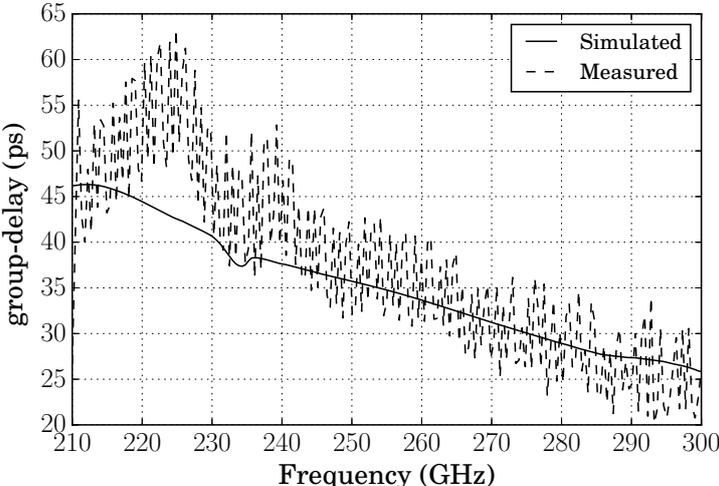
Figure 3.15: Hardware correlation for the group-delay variation of the 240 GHz PA. From 220-260 GHz, the simulated group-delay varies only within 34-44 ps. The average measured group-delay matches closely with simulation results from 230 GHz.
