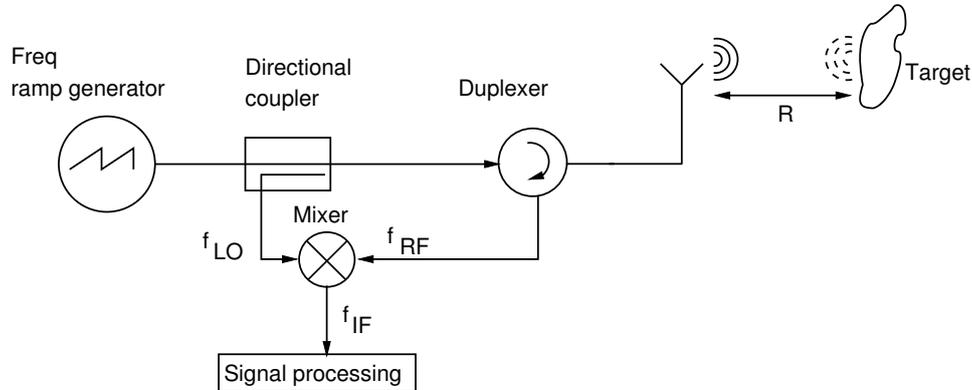
Figure 1.1: Block diagram of a FMCW RADAR system. The down-converted IF signal can be used to estimate the range ( $R$ ) of the target. In general, the higher the bandwidth, the better is the range resolution.
