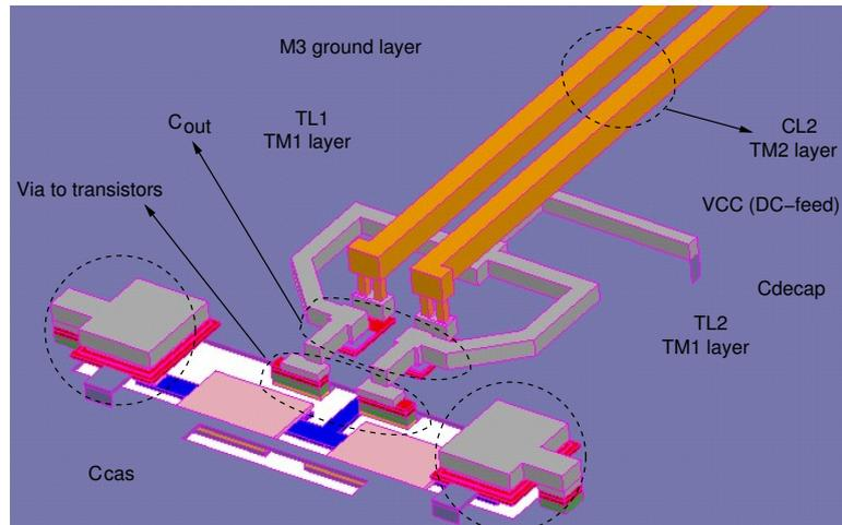
Figure 3.6: 3D model for full EM simulation of the output stage. The via arrays connecting the inductor TL1 to the transistor are approximated as solid metals. The capacitors  $C_{out}$  and  $C_{cas}$  shown in Figure 3.2 are also included in the simulation.
