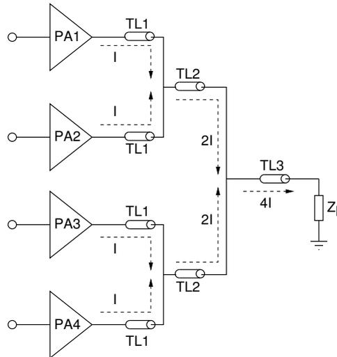
Figure 2.10: Transmission-line based parallel power-combiner. This topology is preferred at mmWave frequencies and higher. The small line dimensions reduce the insertion loss and ensures wideband operation [139, 140].
