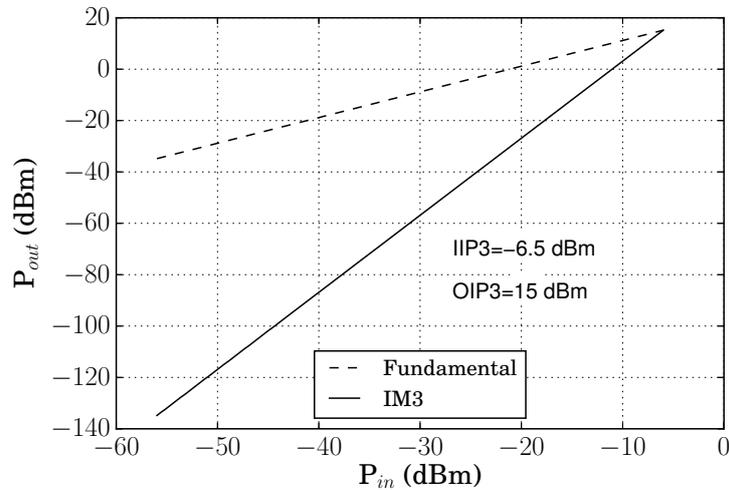
Figure 3.11: Simulated IIP3 of the 240 GHz PA. At 240 GHz, IIP3 is -6.5 dBm and OIP3 is 15 dBm.
