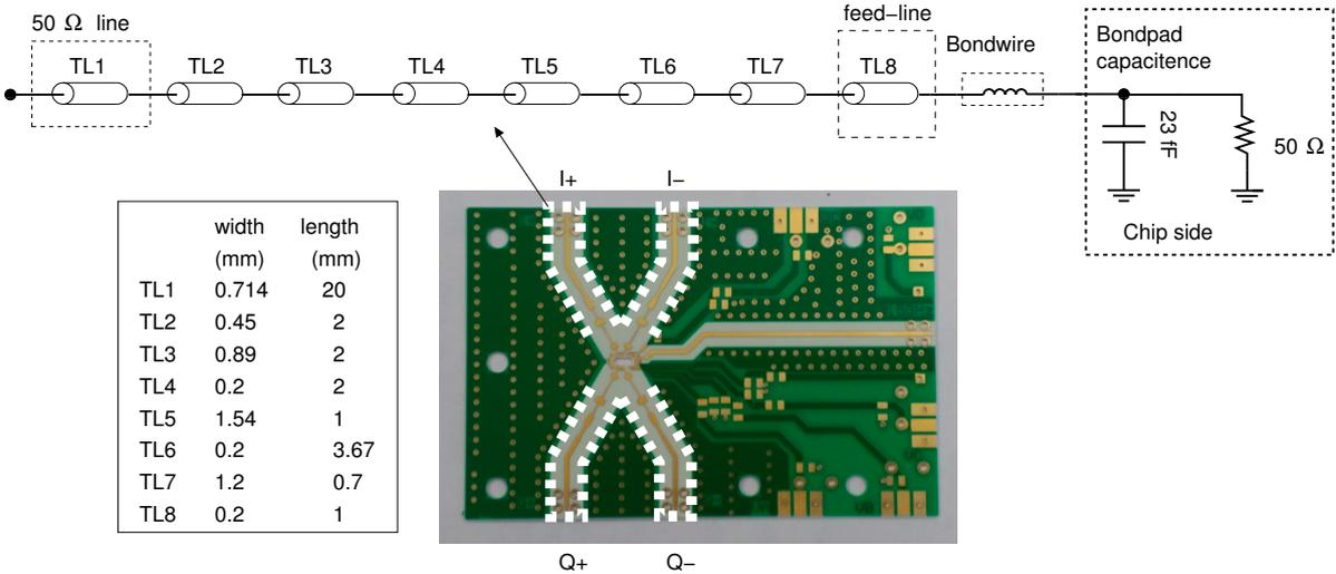
Figure 4.4: Microstrip-line based stepped impedance low-pass filter from the final design iteration in the Rogers 4350B PCB material. For this optimization, wire-bond inductance and feed-lines are included as elements of the filter.
