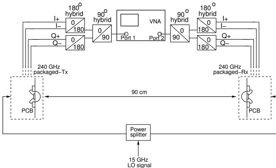
Figure 4.18: Measurement setup for the IF bandwidth characterization of the 240 GHz packaged-Tx and Rx chipset. The Tx and Rx are placed back-to-back over a 90 cm distance. The IF inputs are connected to a VNA using external  $90^\circ$  and  $180^\circ$  hybrids for single-sideband modulation.
