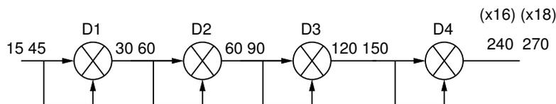
Figure 3.39: The  $3^{rd}$  harmonic component in the input signal (15 GHz) of D1 results in a spurious  $18^{th}$  harmonic at the overall output. The 90 GHz mixing product at the output of D1 is too high for D2, and is hence rejected.
