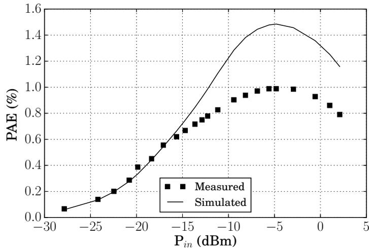
Figure 3.18: Hardware correlation for the PAE measurements of the 240 GHz PA. At 240 GHz, the peak PAE is 1% which is 0.5% less than simulation results.
