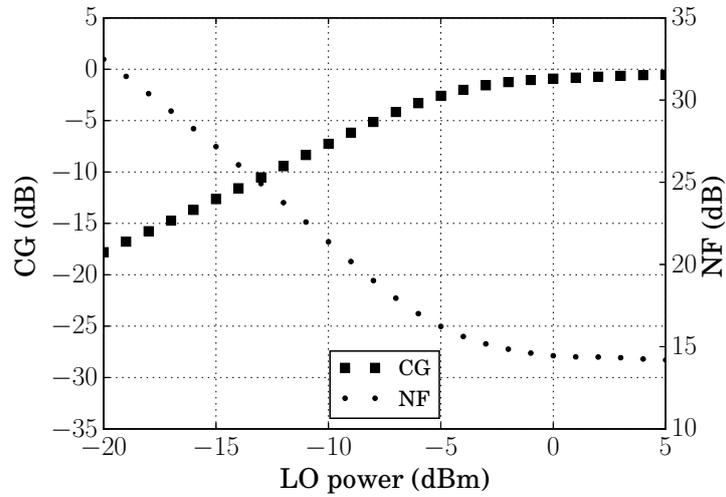
Figure 3.57: Simulation results for the variation of CG and NF of the 240 GHz down-conversion mixer at different LO drive power levels. At an LO frequency of 240 GHz, the optimum LO drive power is greater than -2.5 dBm.
