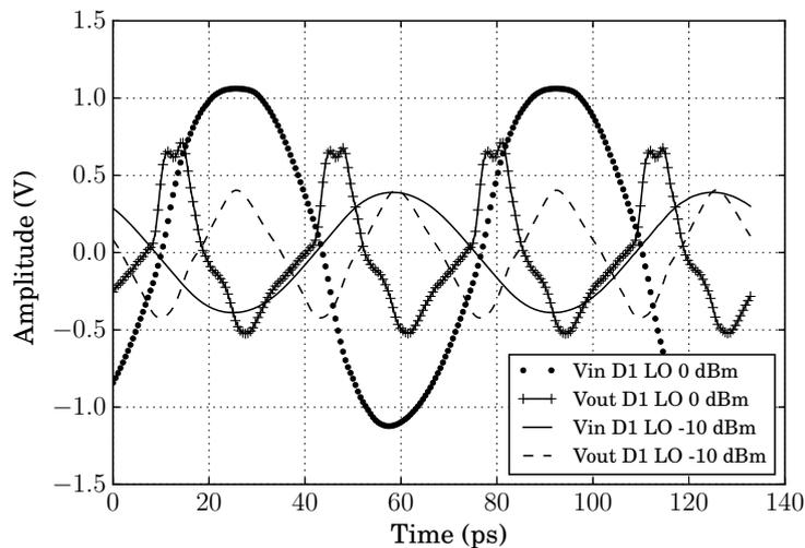
Figure 3.38: Simulated time-domain waveform at the output of the active balun and doubler D1 for an external input LO signal at 15 GHz. As the input power is increased from -10 to 0 dBm, the  $3^{rd}$  harmonic component at the output of the balun increases, which results in a distorted waveform at the output of D1.
