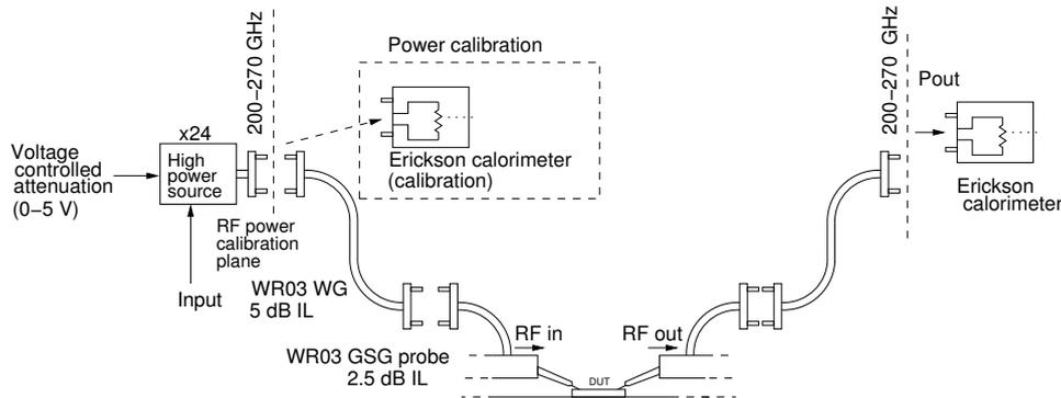
Figure 3.16: Measurement setup for the large-signal bandwidth and linearity characterization of the 240 GHz PA. An external WR03 wideband high power source capable of delivering up to 6 mW at 240 GHz is used at the input.
