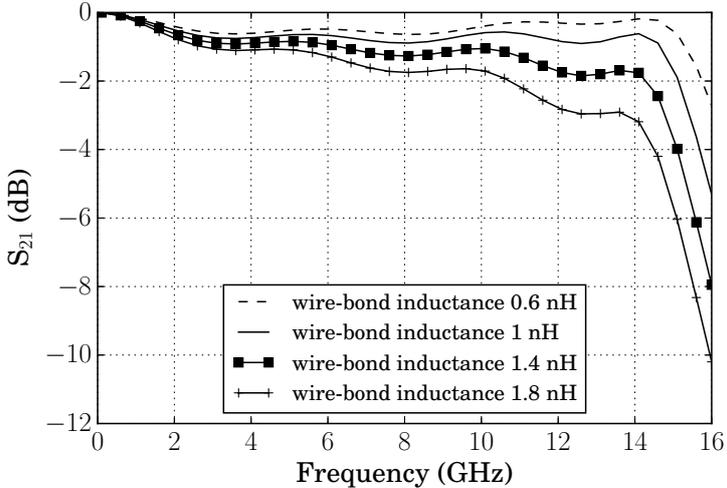
Figure 4.5: Simulated 3-dB bandwidth of the stepped impedance low-pass filter shown in Figure 4.4. The 3-dB bandwidth decreases from 16 to 14 GHz as the wire-bond inductance increases from 0.6 nH to 1.8 nH, and ringing in the passband is eliminated.
