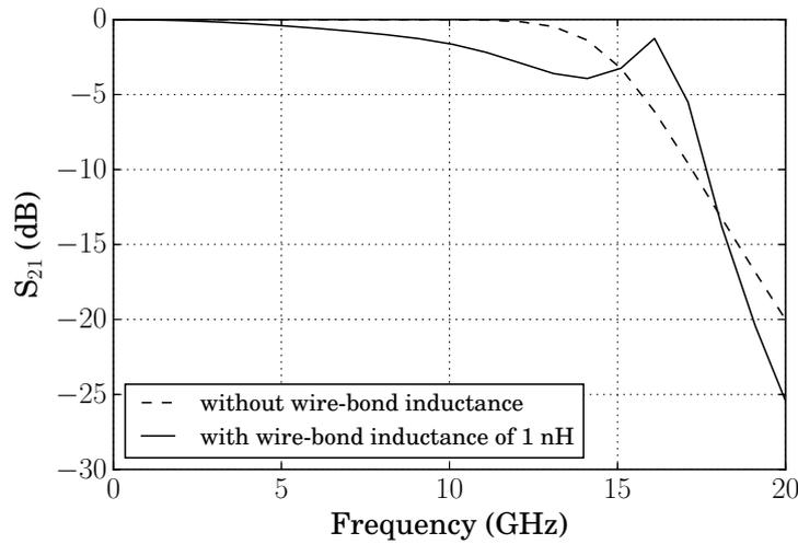
Figure 4.3: Simulated 3-dB bandwidth of the ideal lumped LC low-pass filter is 15 GHz without the wire-bond inductance. A wire-bond inductance of 1 nH reduces the bandwidth and introduces a gain ripple of 3-dB at the passband edges.
