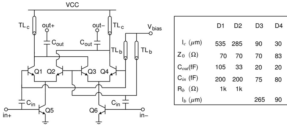
Figure 3.34: Schematic of the unit frequency doubler stage. The inductances  $TL_b$  and  $TL_c$  are implemented as shielded microstrip-lines in the TM2 metal layer with lengths  $l_b$  and  $l_c$  respectively. The capacitor  $C_{in}$  ac-couples the input signal to the switching quad and the transconductance stage. The doublers D1 and D2 are biased using the resistors  $R_b$  instead of  $TL_b$  to save chip area [7, 88].
