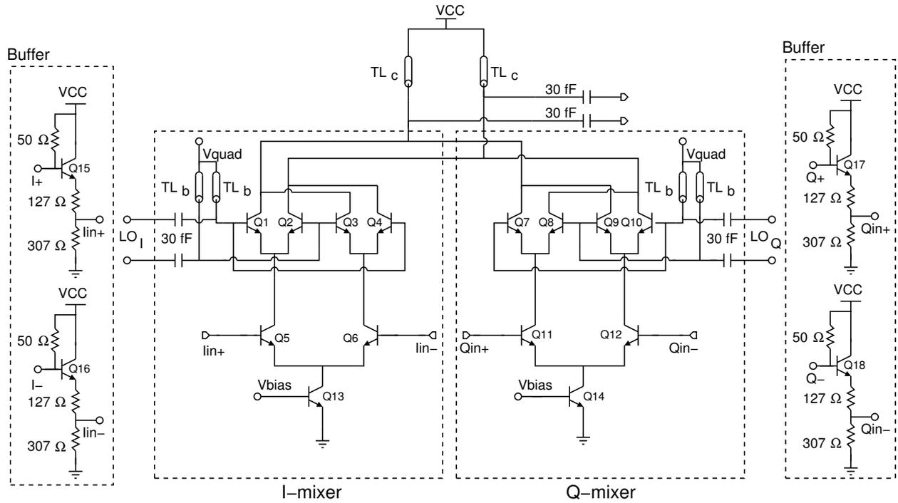
Figure 3.49: Schematic of the 240 GHz quadrature up-conversion mixer. The transistors Q1-Q4 (I-mixer) and Q7-Q10 (Q-mixer) are part of the switching quads, and Q5-Q6 (I-mixer) and Q11-Q12 (Q-mixer) are part of the transconductance stage. At the IF inputs, common-collector based buffer amplifiers with shunt  $50\ \Omega$  resistances are used for wideband matching.
