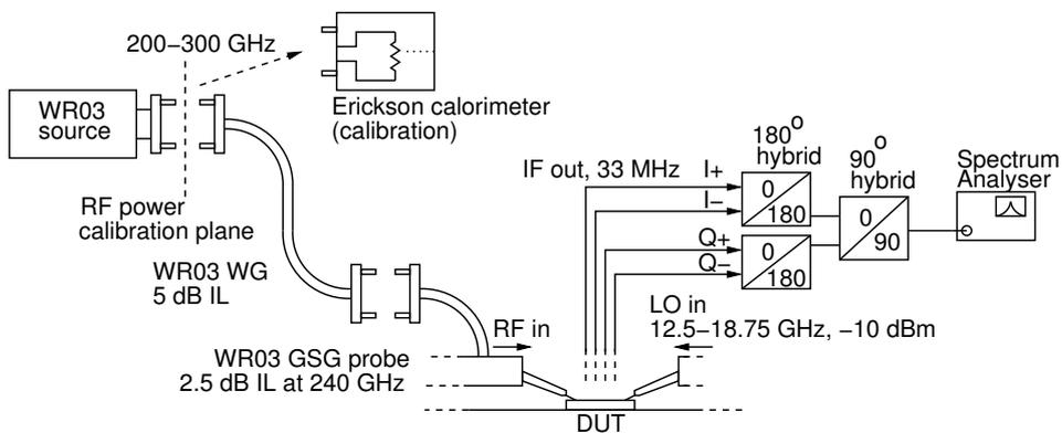
Figure 4.11: Measurement setup for the on-wafer characterization of the Rx. A GSG probe (DC-40 GHz) with a 2.9 mm K-connector is used to couple the external LO signal to the chip. A WR03 GSG probe is used at the Rx input.
