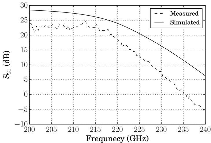
Figure 3.30: Hardware correlation for small-signal bandwidth characterization of the 200-225 GHz combiner-PA. At 213 GHz, the peak gain is 25 dB and the small-signal 3-dB bandwidth is 20 GHz.
