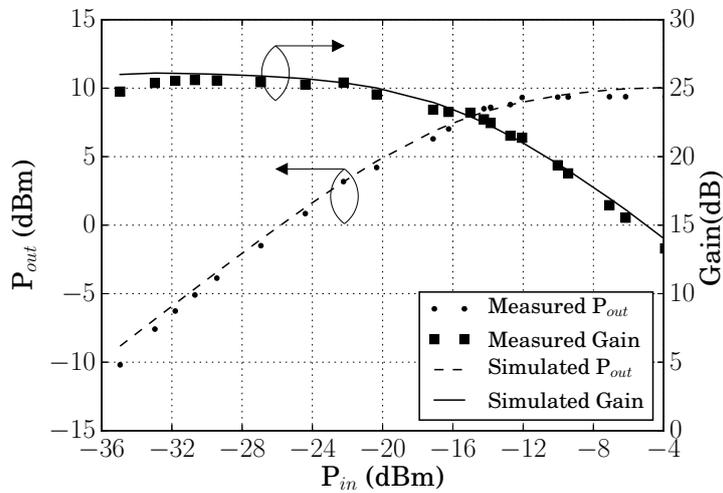
Figure 3.29: Hardware correlation for the linearity characterization of the 200-225 GHz combiner-PA at 215 GHz. The measured  $P_{sat}$  is 9.6 dBm,  $IP_{1dB}$  is -19 dBm and  $OP_{1dB}$  is 5.5 dBm.
