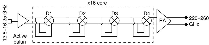
Figure 3.32: Top-level block diagram of the 240 GHz frequency multiplier-based LO signal source [7, 88]. It consists of an active balun, followed by four cascaded frequency doubler stages (D1-D4) and a three-stage 240 GHz PA.
