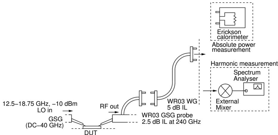
Figure 3.43: Measurement setup for large-signal bandwidth characterization of the 240 GHz LO signal source. The low-frequency input signal (below 20 GHz) from the synthesizer is coupled to the chip using a GSG probe (DC–40 GHz) with a 2.9 mm K-connector. The output signal is measured using a WR03 GSG waveguide probe using an Erickson calorimeter and harmonic mixer.
