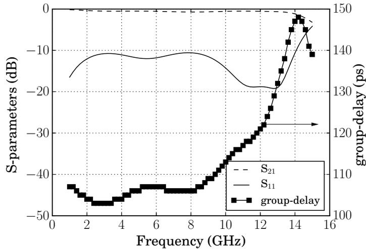
Figure 4.7: Simulation results from the full-EM simulation of the PCB filter. The  $S_{21}$  in the passband is -0.5 dB, 3-dB bandwidth is 15 GHz and  $S_{11}$  is less than -10 dB up to 14 GHz. The group-delay variation is less than 10% up to 9 GHz.
