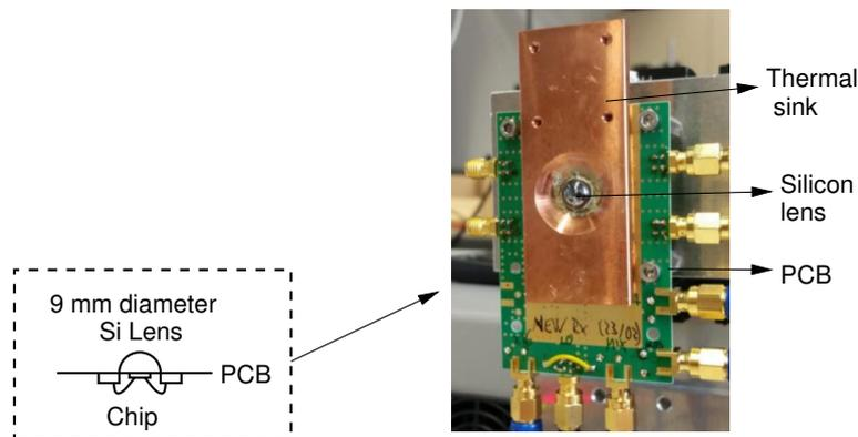
Figure 4.8: Lens-mounted 240 GHz packaged-Tx. The chip is glued to an external silicon lens with a diameter of 9 mm and wire bonded onto a low-cost PCB material (ROGERS 4350B). The 240 GHz packaged-Rx looks similar and is not shown here.
