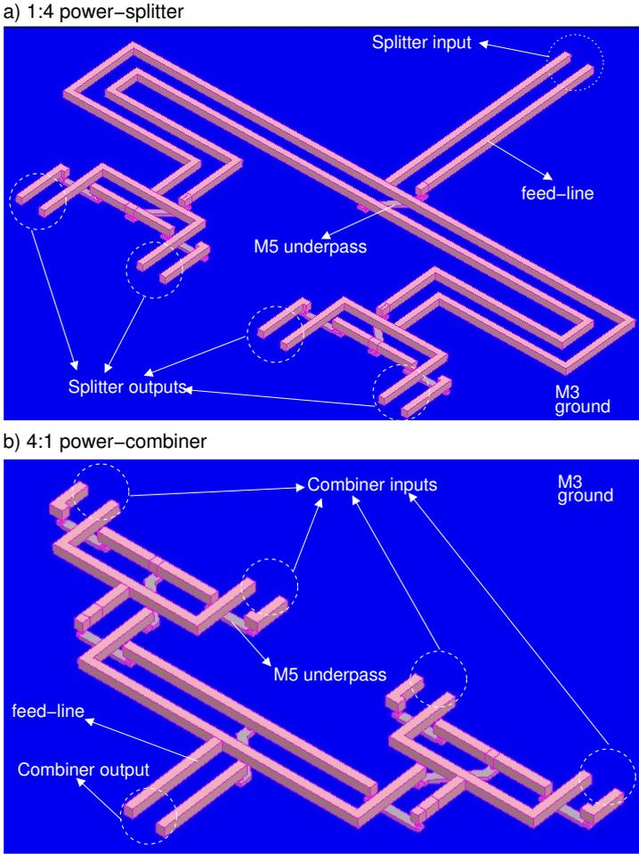
Figure 3.24: 3D-model for full EM simulation of a) 1:4 power-splitter, and b) 4:1 power-combiner in HFSS. At the input and output, wave-ports are defined (not shown here) for higher accuracy.
