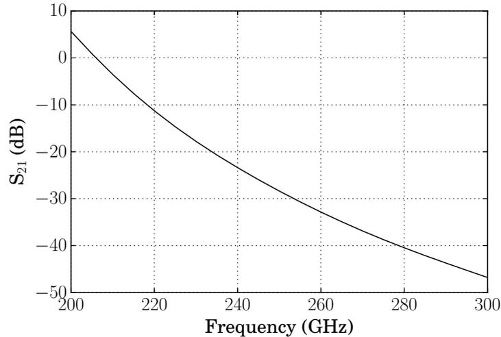
Figure 3.10: Simulated small-signal common-mode gain of the 240 GHz PA. The attenuation is higher than 15 dB above 225 GHz. This makes the design robust against parasitic common-mode oscillations.
