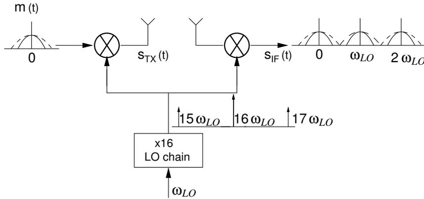
Figure 3.33: Effect of spurious LO harmonics on the down-converted IF signal for coherent detection. For this illustration, only the spurious 15<sup>th</sup> and 17<sup>th</sup> harmonics were considered to simplify the analysis.
