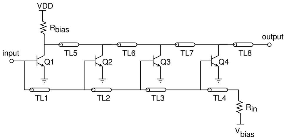
Figure 2.3: Schematic of a distributed amplifier. The overall amplifier architecture is additive, which results in wideband operation from DC to very high frequencies.
