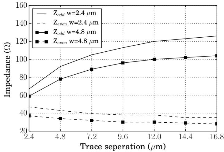
Figure 3.21: Simulated  $Z_{odd}$  and  $Z_{even}$  versus trace-separation  $s$  for coupled microstrip-lines on the M6 metal layer of the BEOL. For this design,  $s=7 \mu\text{m}$  is optimum. For  $w=2.4 \mu\text{m}$ , this corresponds to a  $Z_{odd}$  of  $105 \Omega$  and  $Z_{even}$  of  $38 \Omega$ .
