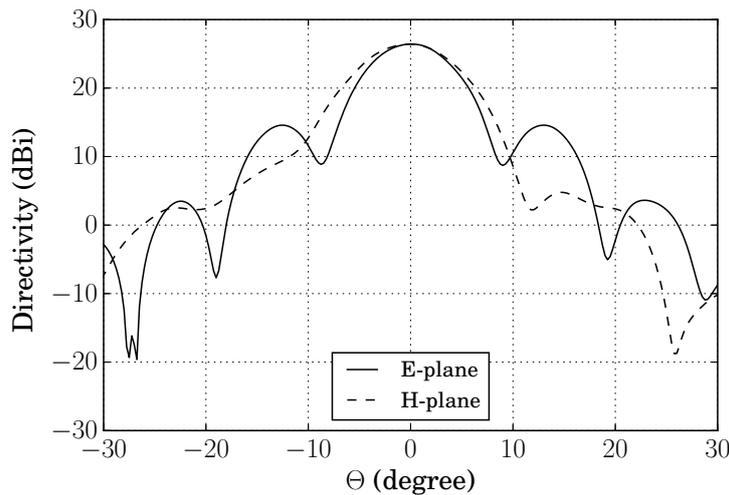
Figure 4.17: Measured directivity of the on-chip antenna of the 240 GHz packaged-Tx and Rx. The FWHP is  $\pm 4^\circ$  in the E-plane and  $\pm 4.5^\circ$  in the H-plane, and this yields an estimated directivity of 26.4 dBi at 240 GHz.
