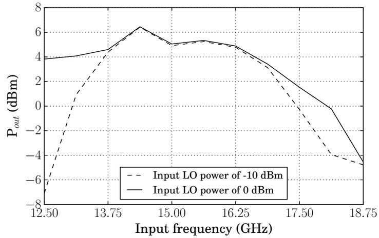
Figure 3.44: Absolute power measurement of the 240 GHz LO signal source. For an input LO power of -10 dBm, the peak output power is 6.4 dBm at 230 GHz, and the 3-dB RF bandwidth is 50 GHz (215-265 GHz). For an input LO power of 0 dBm, the output power remains constant below 13.75 GHz.
