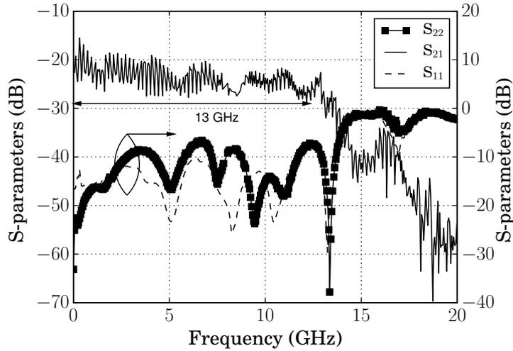
Figure 4.19: Measurement results from the IF bandwidth characterization at a carrier frequency of 240 GHz. This measurement is performed over a wireless link of 90 cm, and the 6-dB IF bandwidth is 13 GHz.
