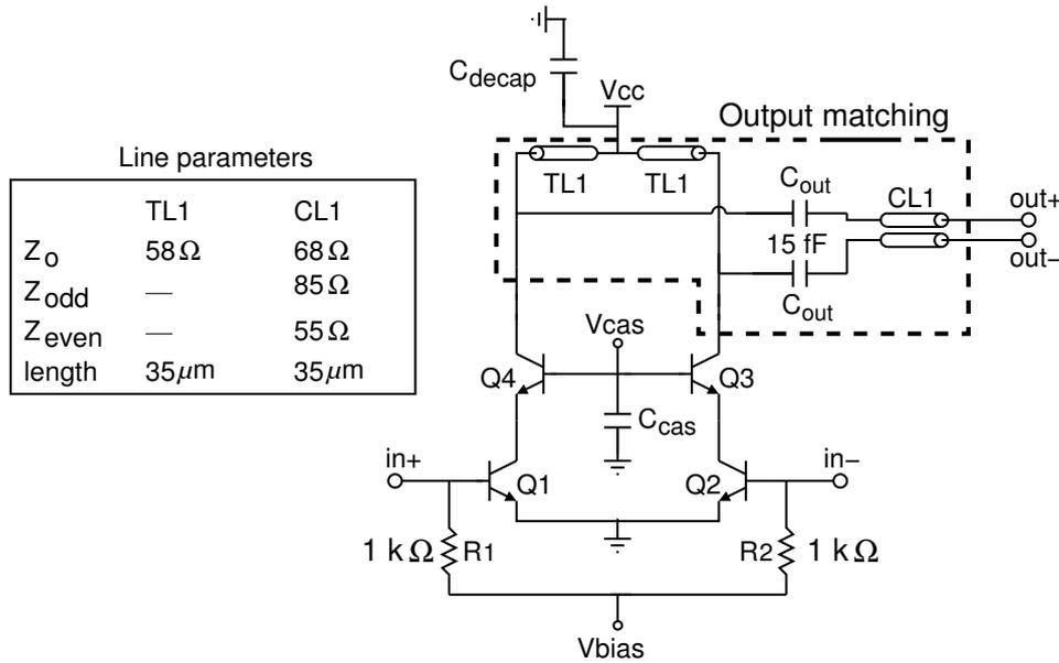
Figure 3.2: Schematic of the output stage of the 240 GHz PA. The transistors Q1-Q4 have an emitter area of  $8 \times (0.96 \times 0.12) \mu\text{m}^2$ . The microstrip-line based inductors TL1, coupled microstrip-line CL1 and the capacitor  $C_{out}$  forms part of the output matching network.
