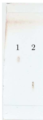
Figure 4.11: Separation of mono- and di-glucosides; silica-gel 60 F_{254} TLC plate, eluted by \text{CHCl}_3/\text{MeOH} (8/2) and visualised by \text{H}_2\text{SO}_4 (200 g/L). (1) \text{C}_{12} - \beta -D-glucopyranoside; (2) \text{C}_{12} - \beta -D-maltoside
