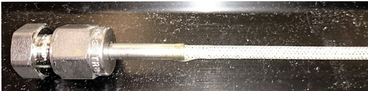
FIGURE 94: Development of the carbon fibre pipe filled with diamond powder-cyanate ester resin
