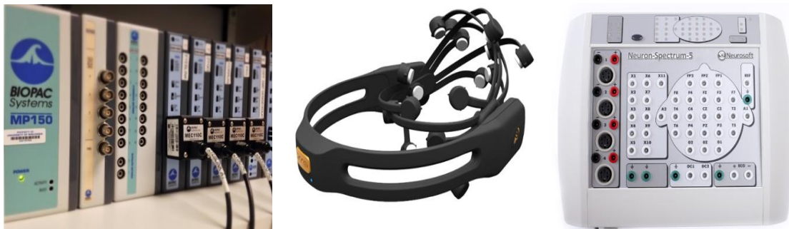
Figure 2.3.1 EEG devices - BIOPAC MP150 (L), Emotiv EPOC Headset (M) and Neuron-Spectrum-5 (R)
