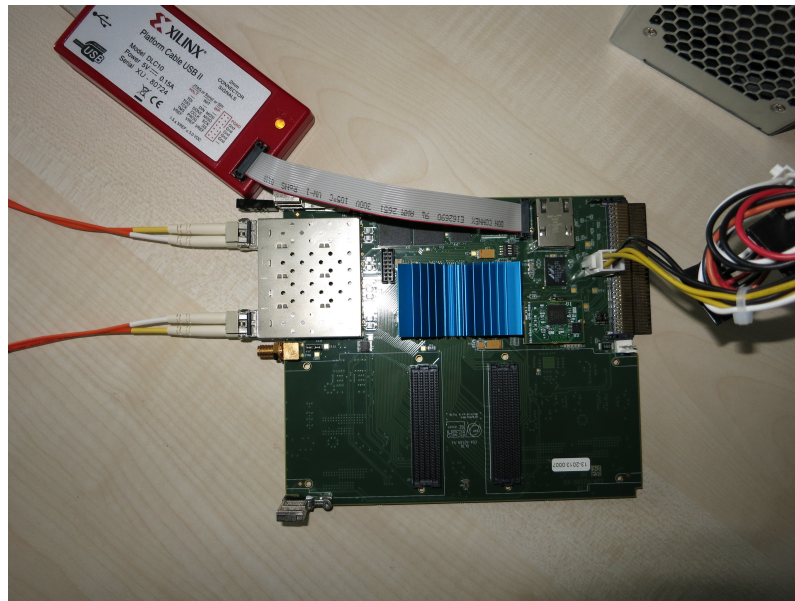
Figure 10.7: Picture of the GBT Link Interface Board for evaluating the GBT firmware.
