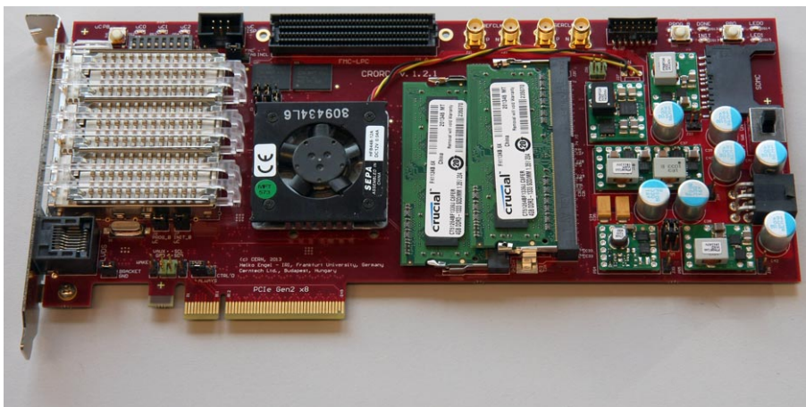
Figure 4.12: Picture of the latest ROBIN card receiving the detector data in the ROS-PCs
