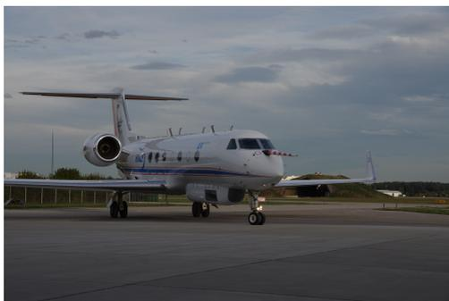
**Figure 7.1:** The German High Altitude and Long range research aircraft (HALO) on the runway. The GLORIA instrument is mounted in the belly pod.
