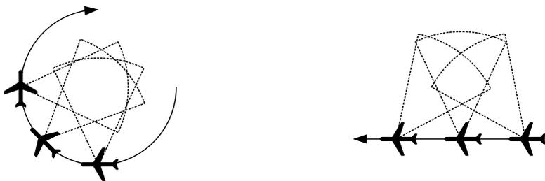
**Figure 2.3:** Schematics of 3-D tomographic flight paths (*Ungermaun*, 2011). Left: Closed loop circular flight pattern. Right: Linear flight path with panning.
