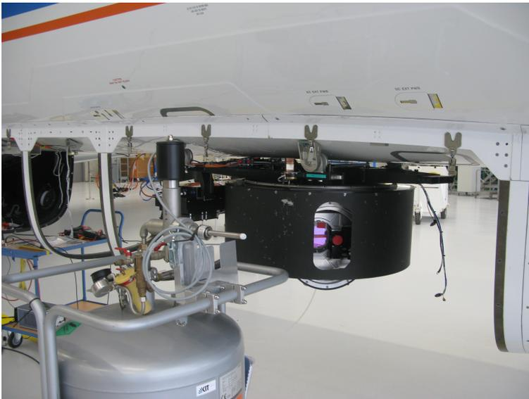
**Figure 2.4:** The GLORIA instrument mounted in the belly pod of the German High Altitude Long Range Research Aircraft.
