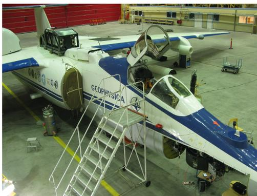
**Figure 5.1:** The Russian M-55 Geophysica high altitude research aircraft during integration of the scientific instruments for ESSenCe. GLORIA is mounted in the front bay.
