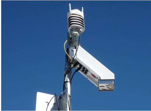
Figure 6.7: Picture of the weather station deployed on top of the CRS. Weather sensor (top) and field mill (bottom).
