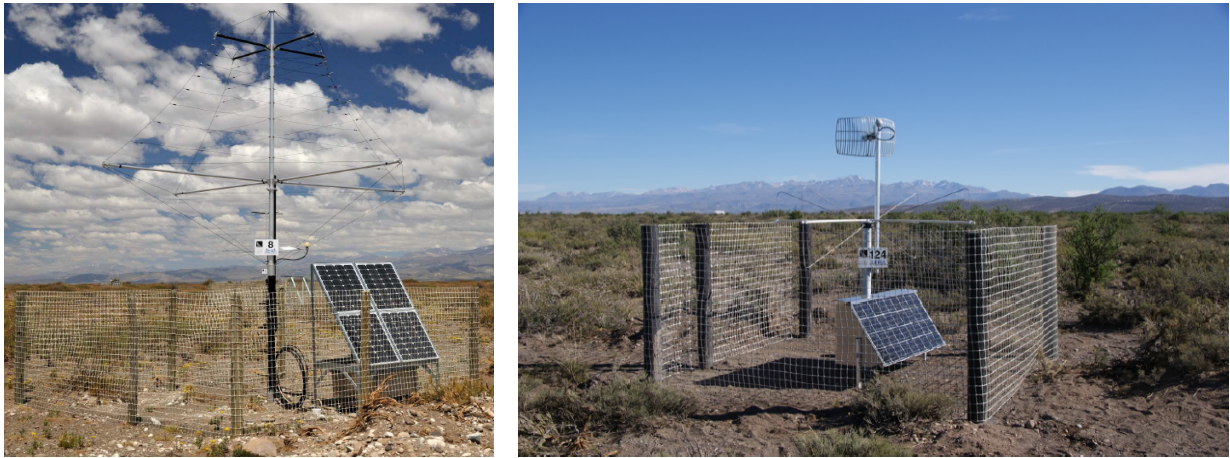
Figure 6.4: Pictures of a phase I station with the LPDA (left) and a phase II/III station with the Butterfly antenna (right) in the Argentinean pampa.
