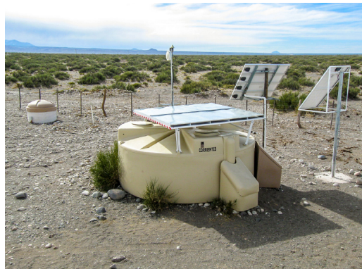
Figure 5.8: Picture of a water Cherenkov detector with a 4 m 2 scintillation prototype detector placed on top.
