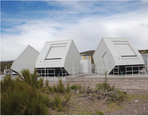
Figure 5.6: Picture of the three HEAT telescopes with closed shutters tilted to the upward mode.
