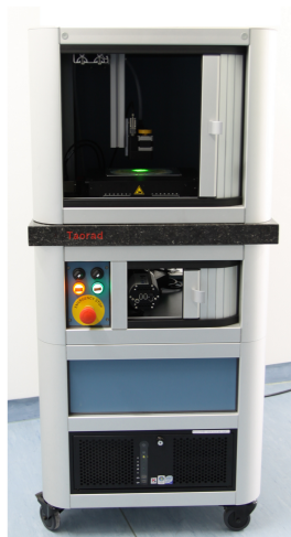
Figure 3.1: Employed polarimetric setups. A) Large-area polarimeter and B) polarizing microscope. The polarization elements alter the polarization state of the light in a defined manner. The large-area polarimeter additionally contains a tilting object stage and the polarizing microscope a moveable object stage to enable a successive scanning of the tissue.
