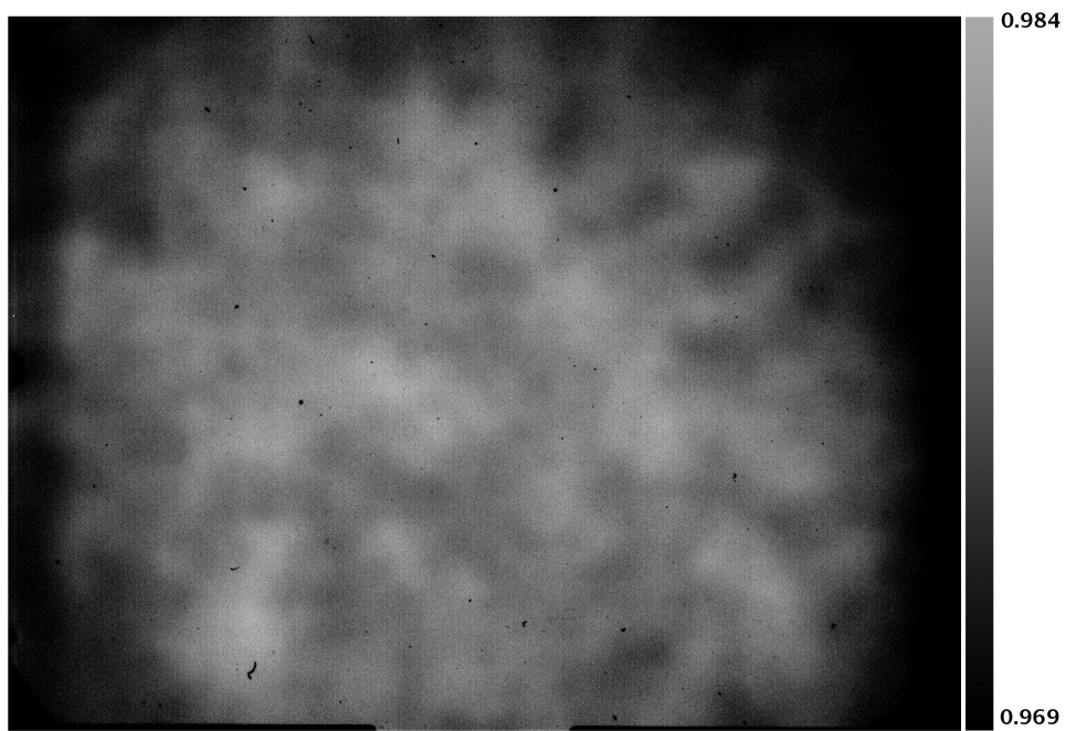
Figure 3.12: Polarization efficiency. Contrast enhanced image of the polarization efficiency of the employed linear polarizers of the LAP.
