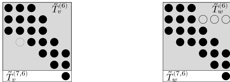
Figure 7.2: Example for the sparsity patterns of the matrices \tilde{T}_v^{(7,6)} and \tilde{T}_w^{(7,6)} as well as \tilde{T}_v^{(6)} and \tilde{T}_w^{(6)} generated by Algorithm 7.1 in case of inexact deflation in step c = 4 in the right Lanczos vector sequence and exact deflation in step c = 5 in the left Lanczos vector sequence for 2 left and right starting vectors. The circles \bullet represent non-zero entries. Empty circles \circ represent entries of small magnitude arising due to orthogonalisation against inexactly deflated vectors. Empty dotted circles \circ represent computed values of small magnitude being the norm of inexactly deflated vectors and are not actually included in the matrices.
