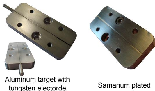
**Figure 3.16:** Picture of the modified aluminum insert to use the tungsten electrodes as photoemissive material (left) and of the samarium-plated target directly after the PVD process (right).
