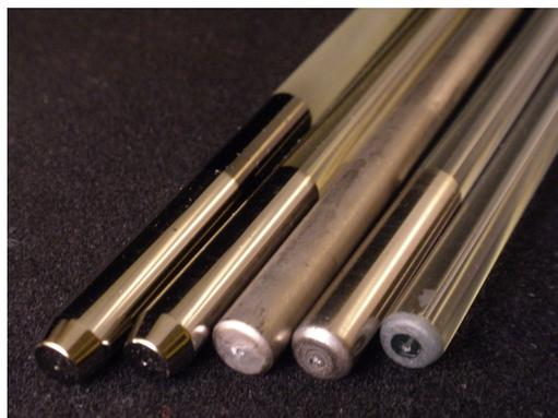
**Figure 3.3:** Different inlet capillaries (f.l.t.r.): Lead oxide coated lead silicate capillary; lead silicate capillary; completely nickel-plated borosilicate capillary; capillary with nickel-plated end caps; borosilicate glass capillary. Picture taken by David Müller [81].
