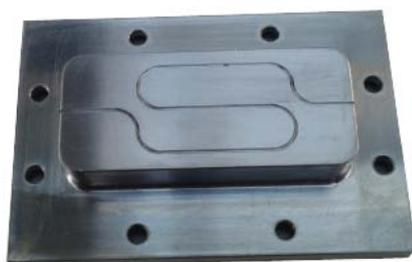
**Figure 3.17:** Picture of the aluminum target with a 2.5-fold increased capillary channel length.
