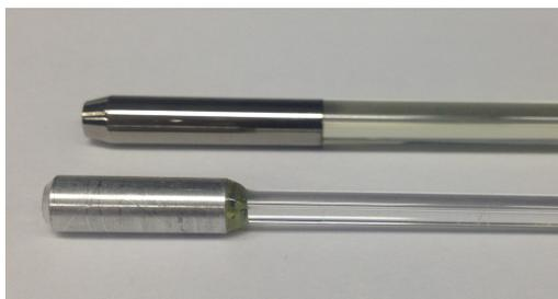
**Figure 3.12:** Photograph of the silica inlet capillary with casing to match the capillary socket in the mass spectrometer and a common Bruker Daltonik inlet capillary made of lead silicate glass.
