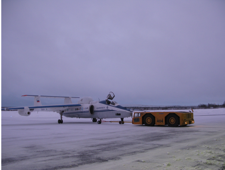
Figure 3.3.: The Myasishchev M55 Geophysica high altitude aircraft deployed during the ESSenCe measurement campaign in 2011. The aircraft is shown being towed back from the runway towards the Arena Arctica hangar at Kiruna Airport, Sweden. The GLORIA instrument is visible behind the opening in the fuselage right below the cockpit.
