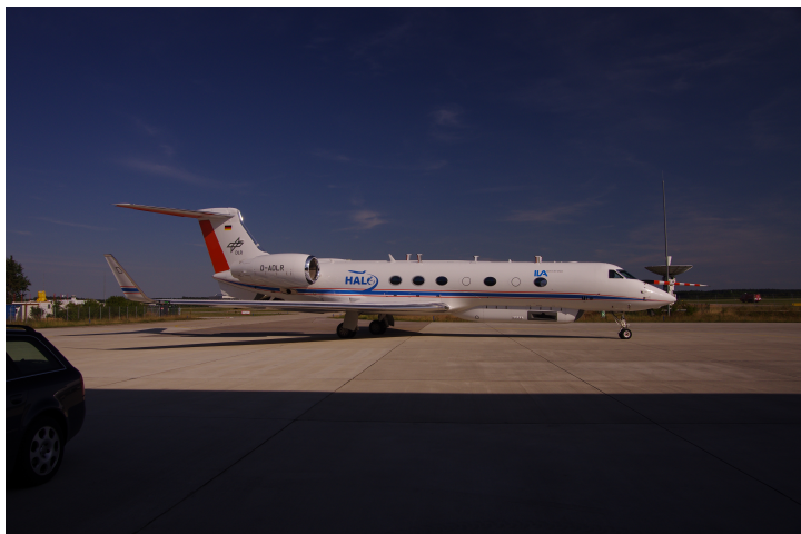
Figure 3.5.: The HALO aircraft, based on the Gulfstream G550 series business jet, was the platform used for the TACTS/ESMVal campaign. The aircraft is operated by DLR and can carry a multitude of instruments, including computing equipment and operating personnel. This figure shows HALO on in front of the DLR flight operations hangar in Oberpfaffenhofen, Germany.
