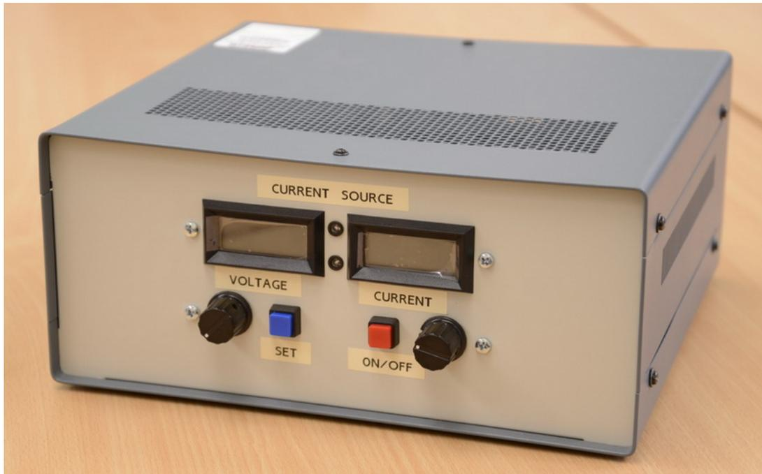
**Figure 6.19:** A picture showing a self-made current source, used for comparison measurements with the commonly used voltage sources, operating with current limitation.
