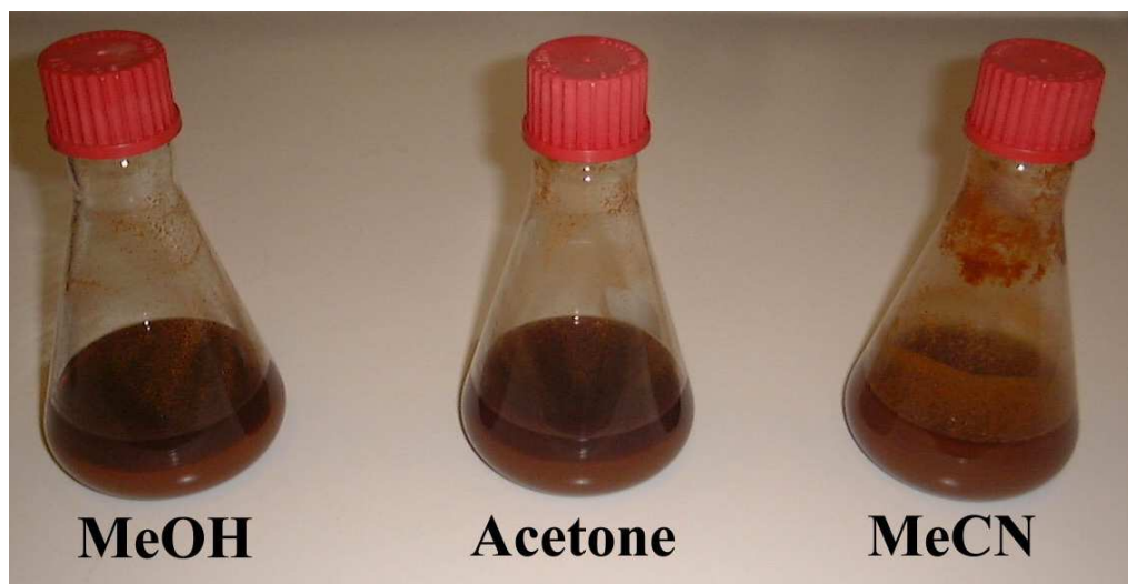
Figure 2.2: Difference in the sedimentation of paprika powder with different extractants
