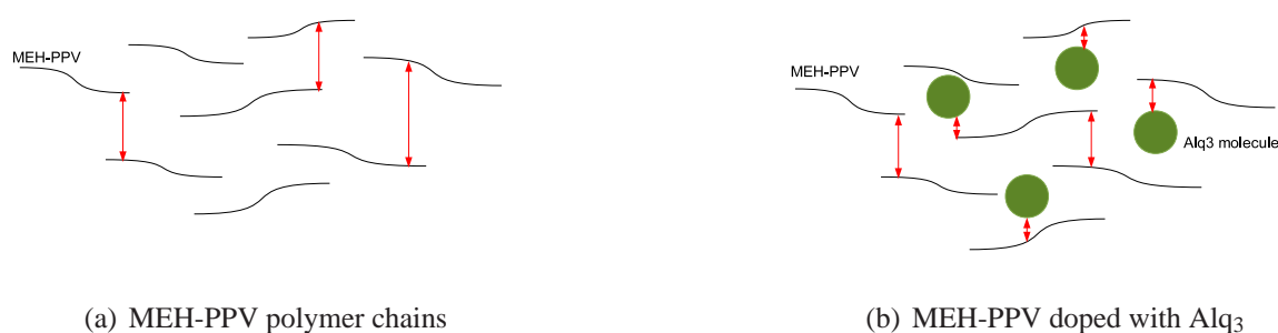
Figure 2.4: MEH-PPV polymer chain with schematically shown interchain energy transfer (a), MEH-PPV doped with \text{Alq}_3 and the corresponding energy transfer between the polymer chain and the molecules.
