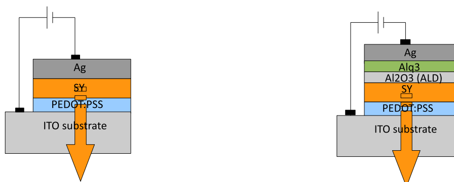
Figure 4.1: reference OLED (left) and investigated multilayer device with a solution processed Alq 3 layer, SY has been protected by a thin aluminum oxide Al 2 O 3 layer deposited by ALD (right)
