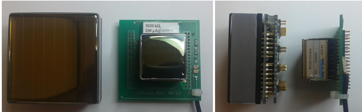
Figure 3.4 – Front (left) and side view (right) of a H8500D-03 with integrated voltage divider and a R11265-103-M16 with home-made voltage divider. The length of the edge is 52 mm for the H8500D-03 and 26.2 mm for the R11265-103-M16.
