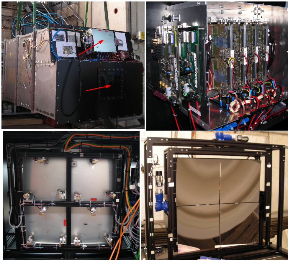
Figure 5.2 – Top: CBM-RICH prototype from the front. The quadratic beam entrance window and the camera housing are marked with arrows (left). Readout electronics (right). Bottom: Mirror tiles mounted on the rotatable frame from back (left) and front (right).
