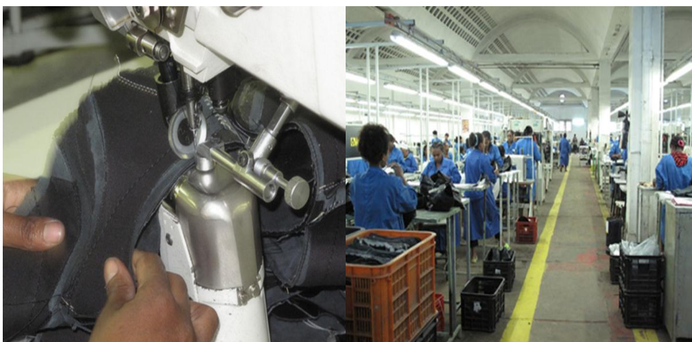
Figure 5. 4 Leather closing/stitching operation: Taken from stitching department of Anbessa Shoe S. Co.
