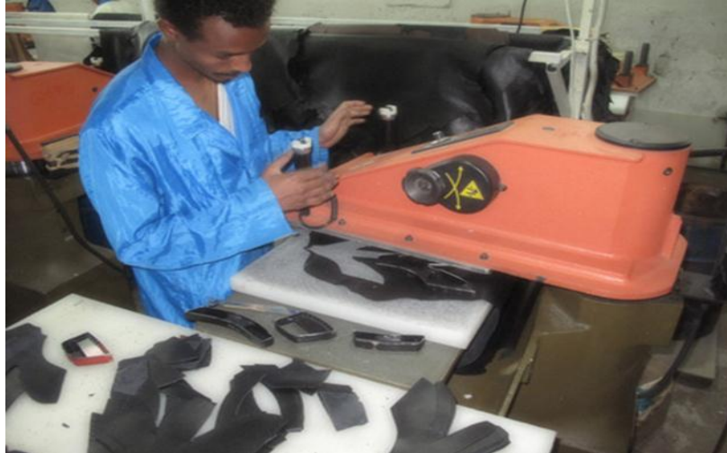
Figure 5. 3 Leather clicking/cutting operation: Taken from cutting department of Anbessa Shoe S. Co.
