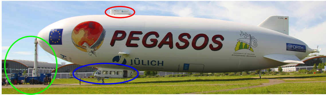
Figure 2.3.: Airship Zeppelin NT as used during the 2012 PEGASOS mission. The Top-Platform is highlighted in red, the gondola including a nose-boom in blue, and the Mast-Truck in green.
