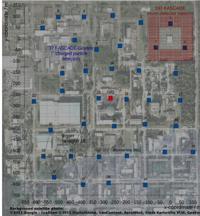
Figure 3.1: Sketch of the setup of the KASCADE-Grande experiment overlaid over a satellite picture of the KIT area (satellite picture taken from [97]). Additionally, the overlaid grid represents the internal KASCADE-Grande array coordinates. See text for further details.
