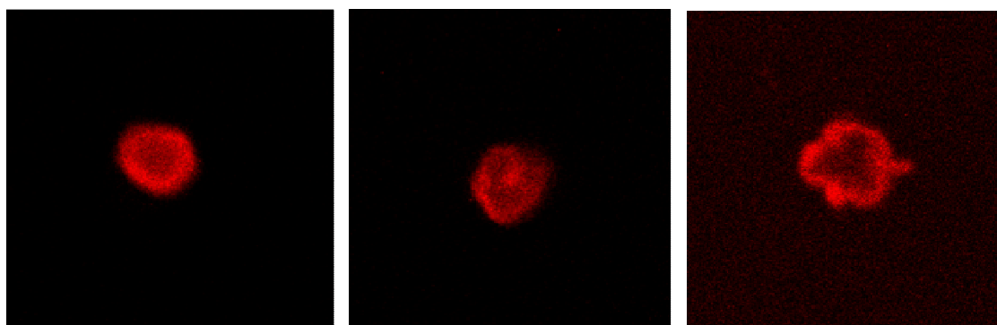
Figure 2.10. Confocal fluorescence microscopy images of three PF2/6- b -P3PyHT (made from precursor A) vesicles in methanolic solution (10 mg/mL) on a glass substrate (vesicle size: 3-4 \mu\text{m} ), left: single vesicle, middle and right: fused vesicles.
