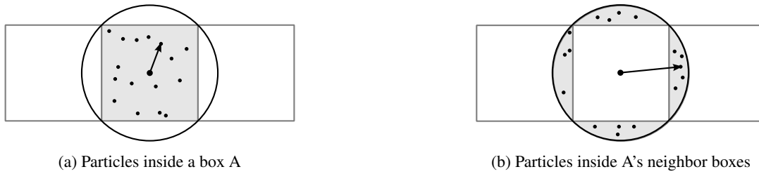
Figure 2.15.: In general it is not possible to set ws to zero, since neighboring boxes may have particles overlapping with the multipole expansion of a neighboring box. However, the convergence of the expansion demands separation. Therefore, next neighbors must not interact via a multipole expansion.
