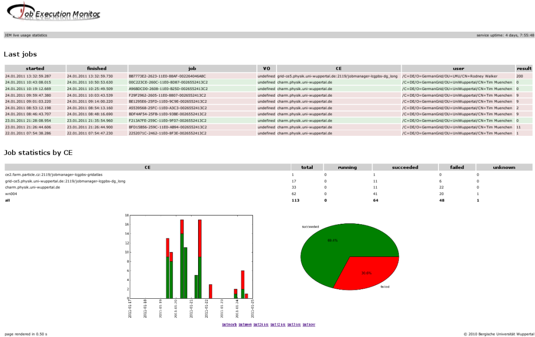
Figure 42: Example of the auto-generated statistics web page, generated by JEM. Shown are the last some job executions with their exit status, as well as statistical plots showing the fractions of succeeded and failed jobs monitored by JEM.
