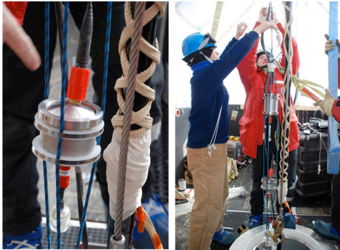
Figure 5.7: Deployment of SPATS string D; stage 6 with HADES B; DS6(2) [Tos pr].
