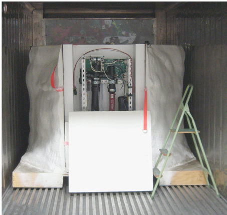
Figure 7.5: IceTop tank with the FCU at the front and with the white thermal isolation coating inside the cooling container [Vog 07].
