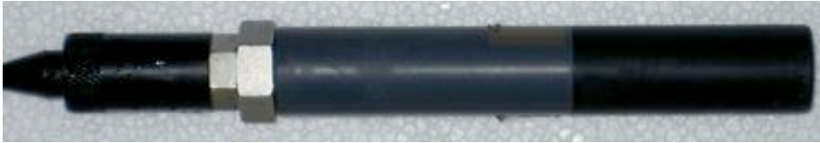
Figure 6.11: Absolutely calibrated hydrophone Sensortech SQ03. The acoustic sensitive area is the black part on the right side.
