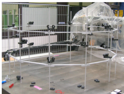
Figure 8.21: The positioning system; three levels equipped with six Murata sensor / transmitter pairs per level [Sch 09].
