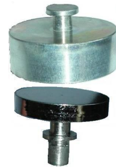
Fig. 5.1: The flat Nb sample with the protection cap.
